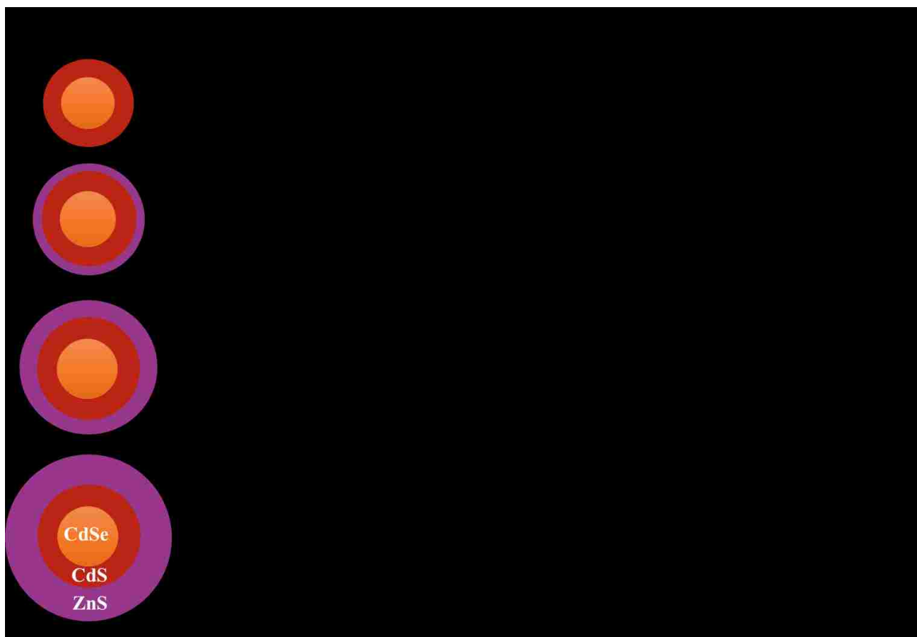
Figure 4.5. (A) Schematic structures of CdSe/CdS/ZnS core/shell/shell QDs with 0, 1, 3, and 5 ML ZnS outer shell. (B) The corresponding 300-s fluorescence traces of the synthesized CdSe/CdS/ZnS under cw laser excitation. (C) Photon counting histograms (PCHs) for the fluorescence traces shown in (B). (D) Zoomed in 20-s fluorescence traces showing the details of the fluorescence blinking behaviors of the QDs.
