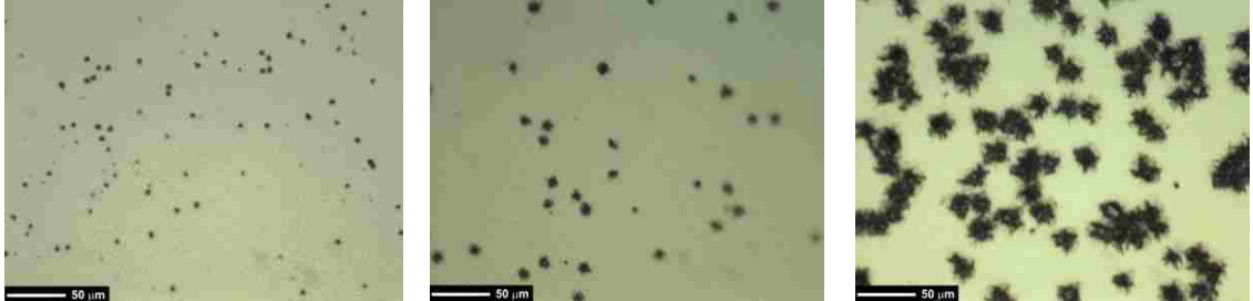
Figure 3.17 Optical microscope images at a magnification of 20X of (a) 5.8 µm, (b) 11.7 µm and (c) 23.3 µm 3C-SiC epitaxial layers showing increased size of protrusion defects at the surface as the epitaxial thickness increases.
