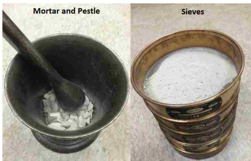
Figure 4: Mortar and pestle were used to grind the rock samples and a series of sieves were used to separate the rock powder to different rock size distributions.
