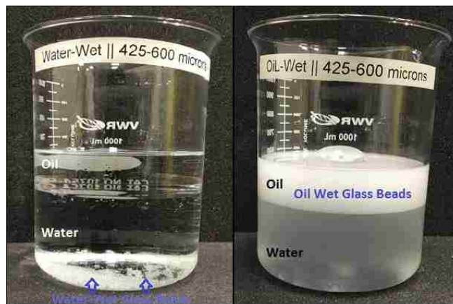
Figure 10: Results of water-wet and oil-wet 425-600 \mu\text{m} glass beads which are in transitional region.
