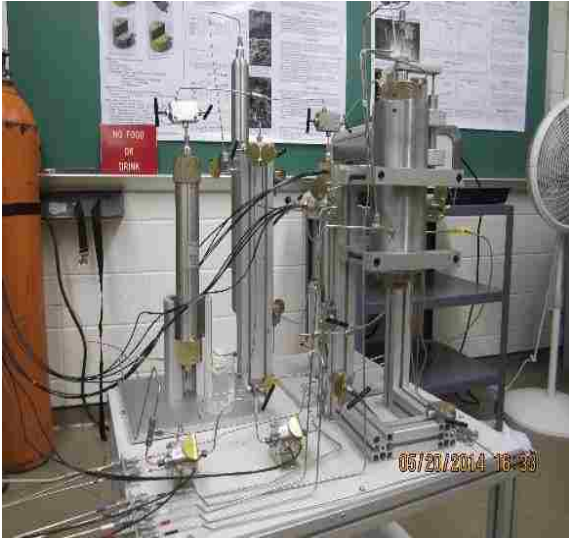
Figure A.1: Core flooding setup showing core holder and instrumentation
