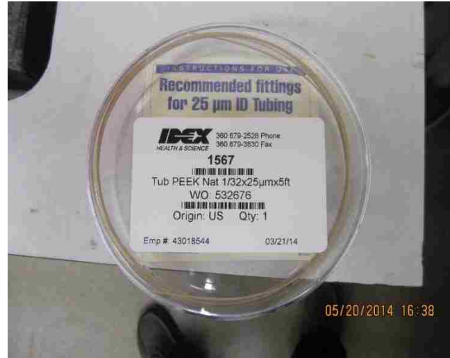
Figure A.6: PEEK micro-tubing used in composite
