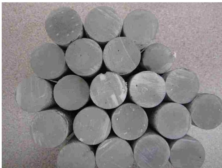
Figure 3.4: Multiple samples of composite core made of kaolinite, cement and polymer PEEK micro-tubes to mimic fractures.
