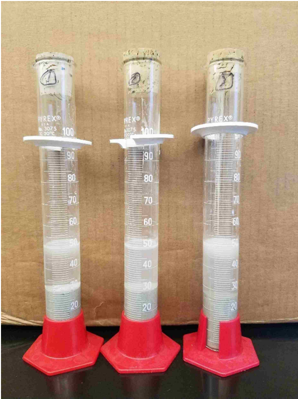
Figure 3.2 ASR expansion test set up. Samples were crated with and without microspheres then cut to be flat then sealed in graduated cylinders shown in a high alkalinity solution. Levels of water and cement were recorded and motored as the cement was cured.
