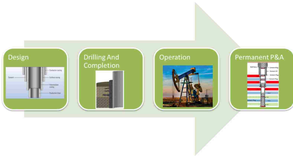
Figure 5.5: Well integrity life line showing show how the design portion of a well must address all other portions of the well life
