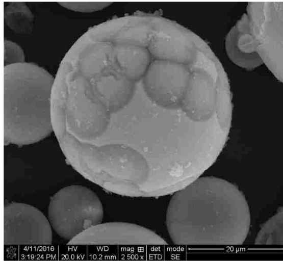
A. SEM image of microsphere after exposure to high alkalinity solution and temperature for one week. Showing initial stage of the reaction where the solution begins reacting with microspheres creation reaction pits on the surface of the microsphere
