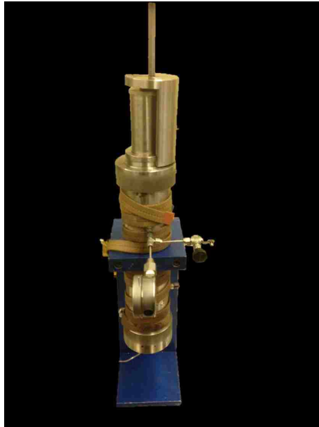
Figure 5.13: Core holder situated vertically for GAGD experiments
