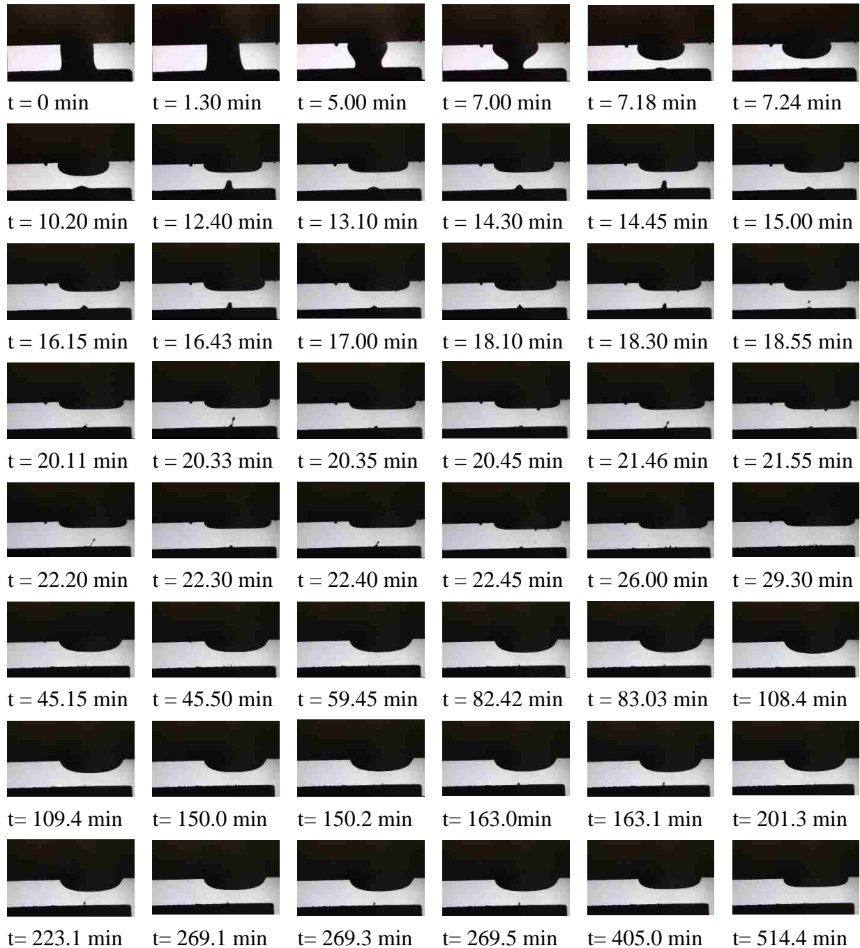
Figure 18: Variation of advancing dynamic contact angle with time during injection of 100 ppm of ALFOTERRA S23-9S 90M.
