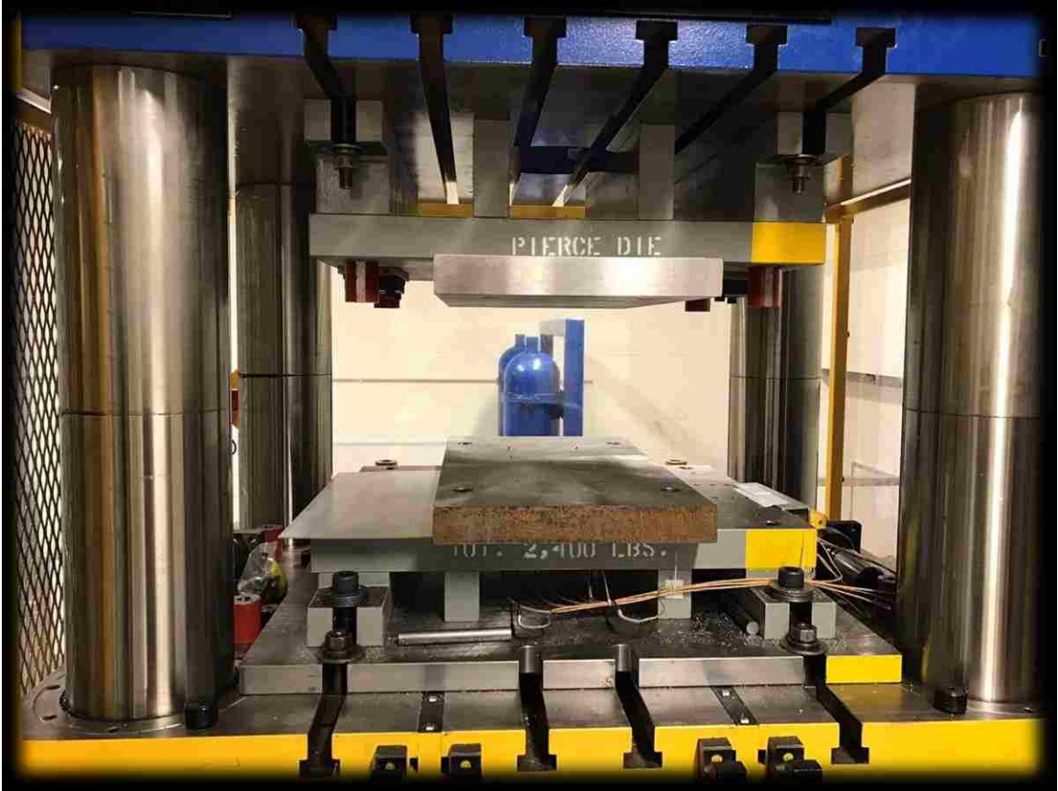
Figure 22 Die plates for quenching
