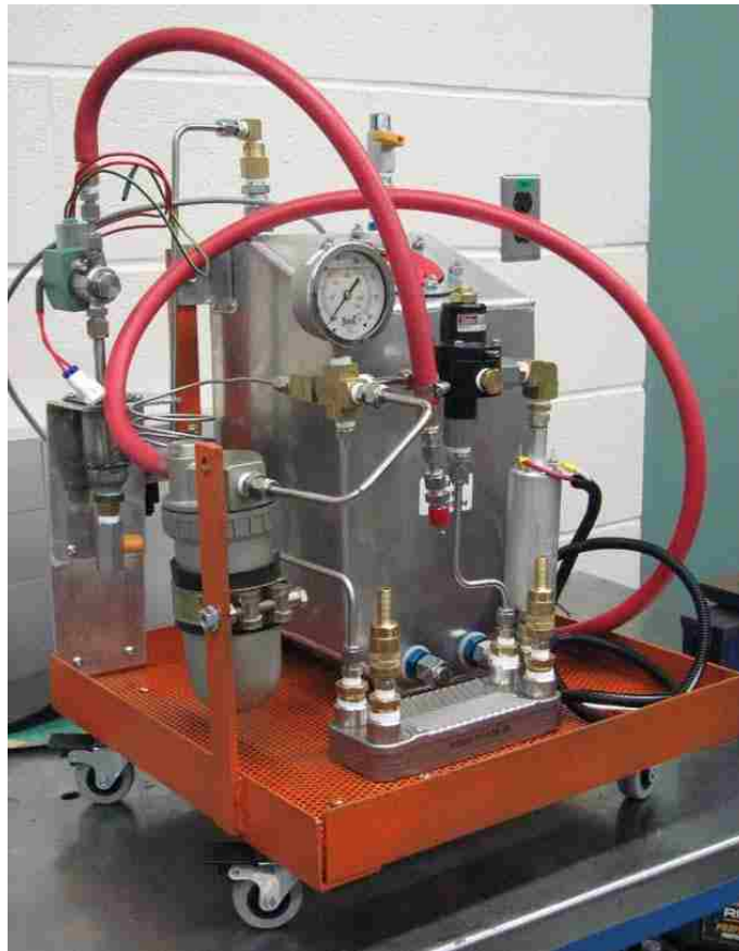
Figure 4-2 PFI Fuel Supply System on Portable Stand
