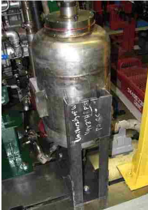
Figure A-3 Stand of the Exhaust Surge Tank
