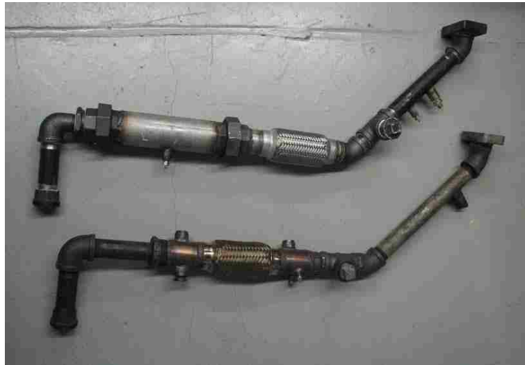
Figure 4-11 Current and Original Exhaust Pipes
