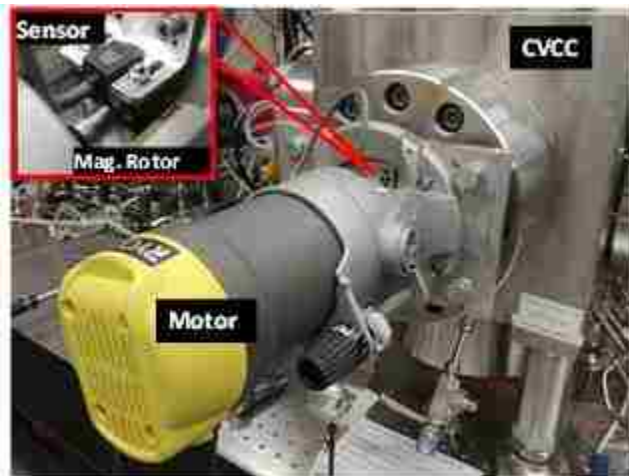
Figure 3-3. Motor for driving fan inside CVCC (Inset: Speed sensor)
