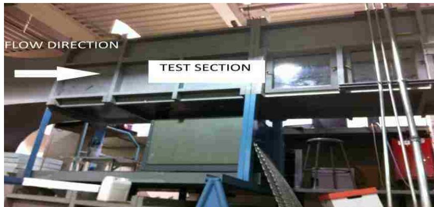
Fig. 3.1. Overall view of the closed loop wind tunnel
