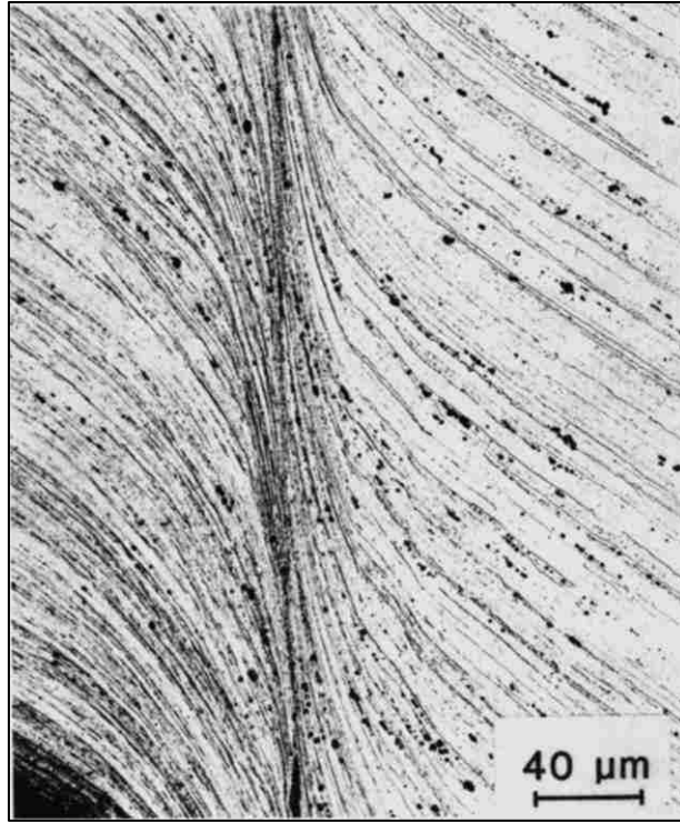
Fig. 2.18. Adiabatic deformed shear band in 7039 aluminum alloy at impact velocity 311 m/s [95].
