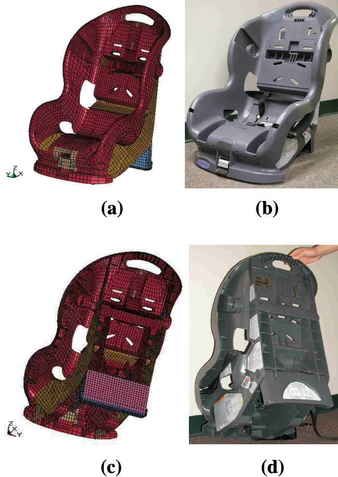
Figure 5-1. Front (a) numerical and (b) actual; Rear (c) numerical and (d) actual view of the deformable Child Restraint System (CRS) [29].
