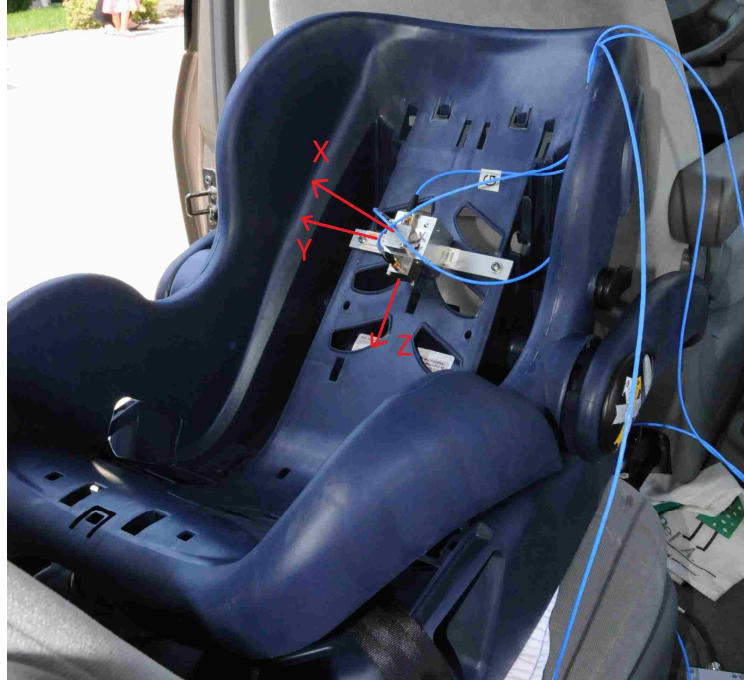
Figure 4-3. The orientation of the accelerometer accordance to SAE J211 standard.
