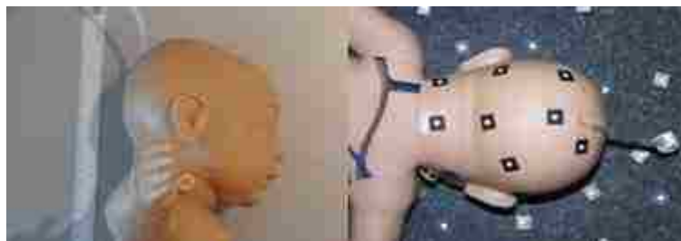
Figure 5-16. Nita Newborn mannequin ready for light scanning.
