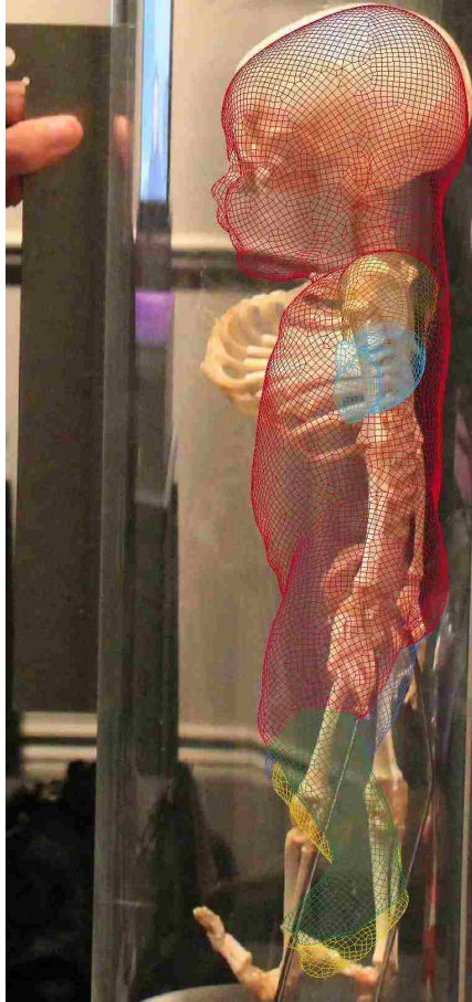
Figure 5-17. The finite element model and the infant skeleton.
