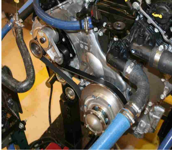
Figure 3.7 - Picture of the start cart BSG system.
