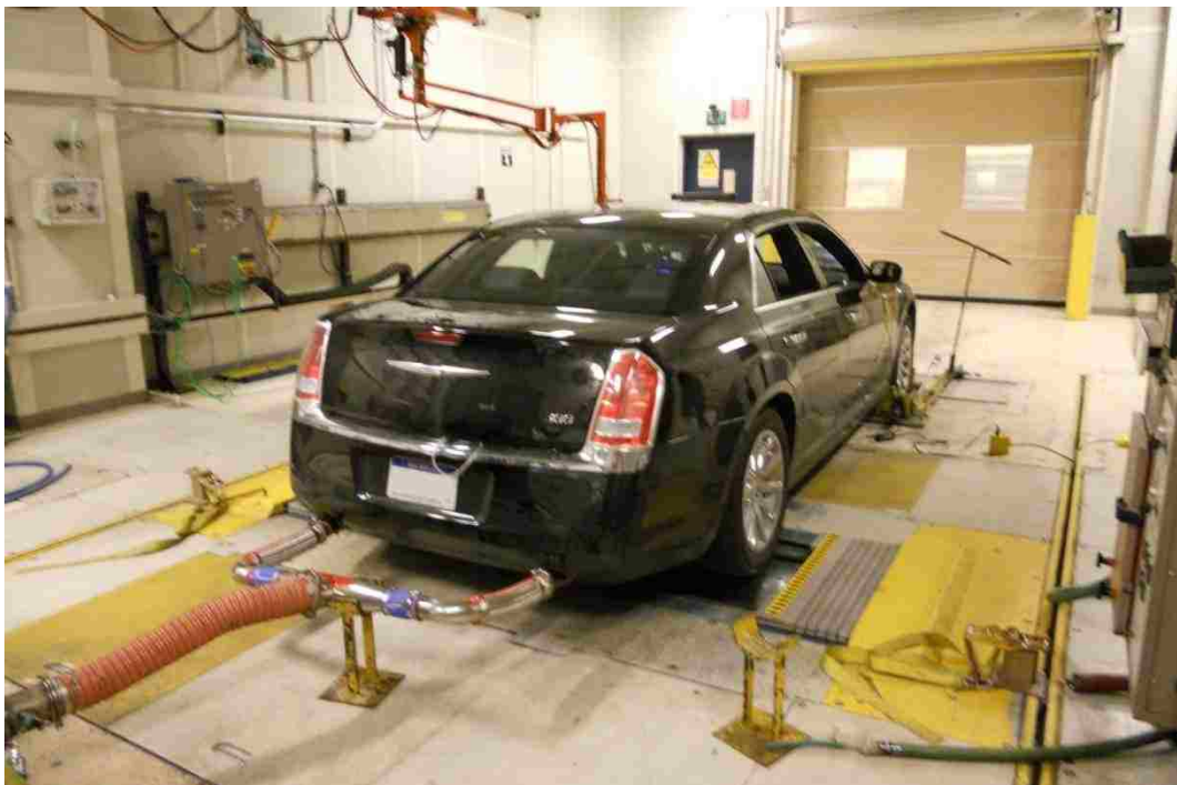
Figure 3.48 - Proof-of-concept test car on the dynamometer. The exhaust collecting hoses can be noticed.
