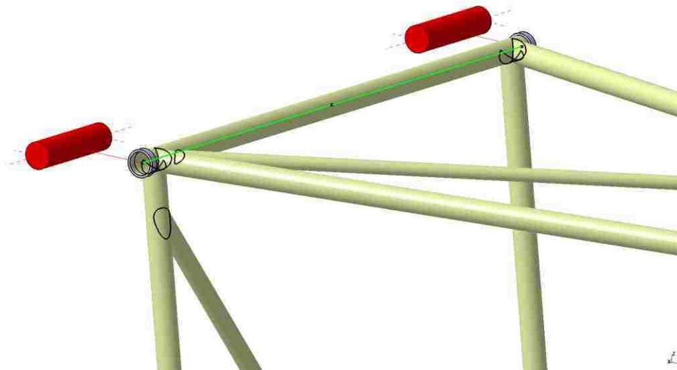
Figure 3.19 Constraint condition for dynamic analysis
