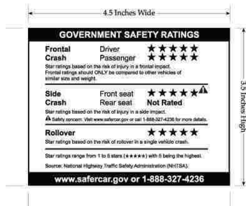
Figure 1.21 Consumer information label for a vehicle with at least one NCAP star rating [22]
