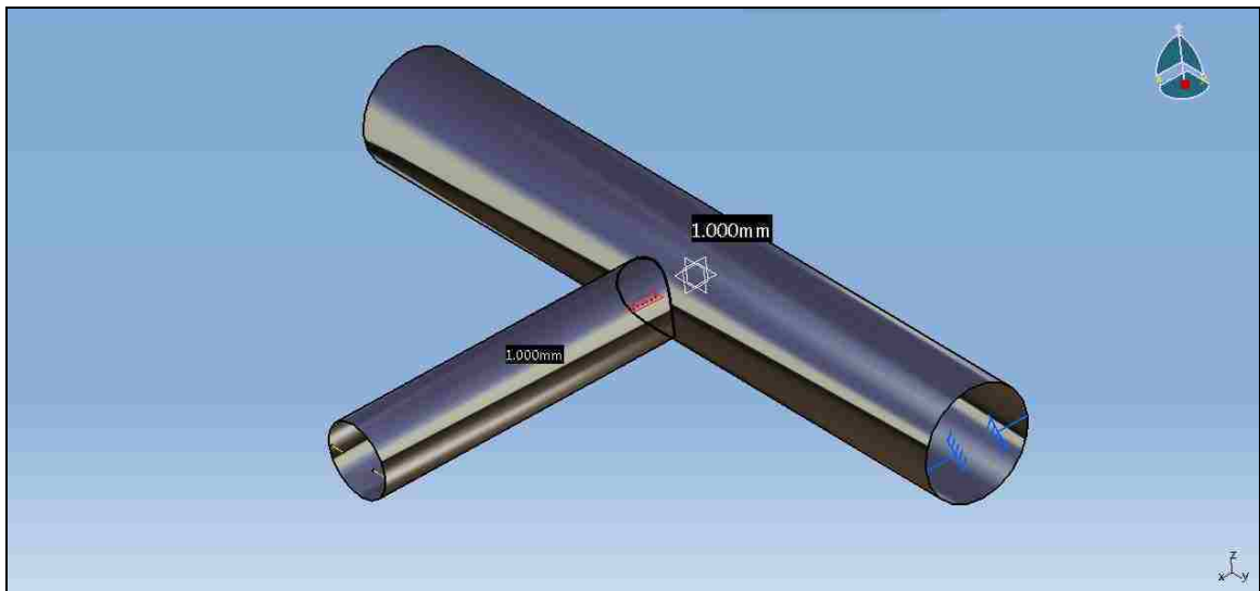
Figure A.1 Seam weld connection tutorial
