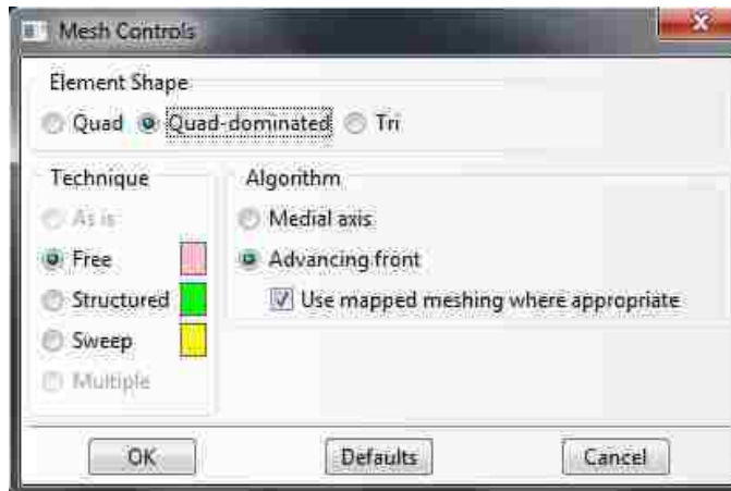
Figure A-11: Mesh control definition in terms of shape, technique and algorithm
