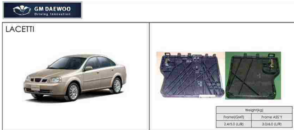
Figure 2-56: Rear seat back solution for Daewoo Lacetti [18]
