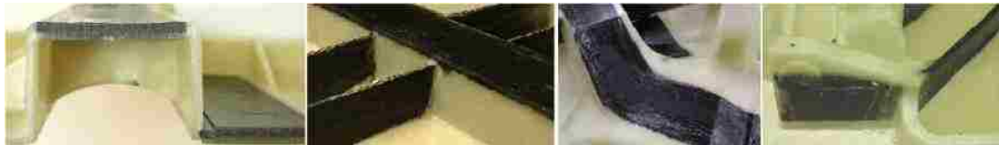
Figure 2-28: Endless fibers application as reinforcement along main load path [11]
