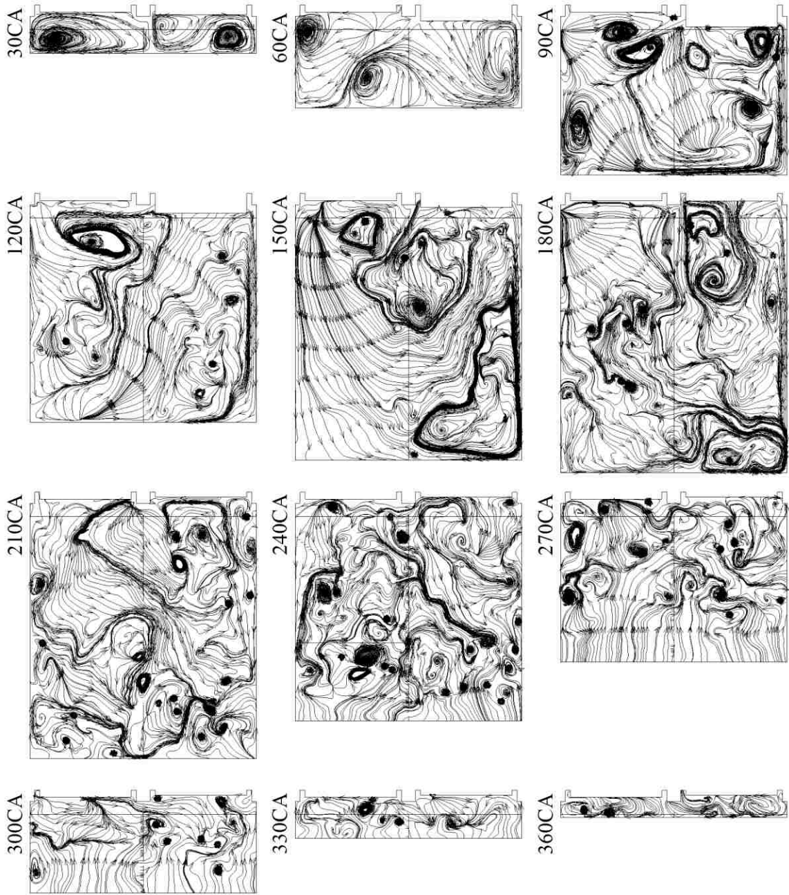
Figure A.8 – Naturally aspirated in-cylinder flow structure development by the DES Spalart-Allmaras model with fine mesh
