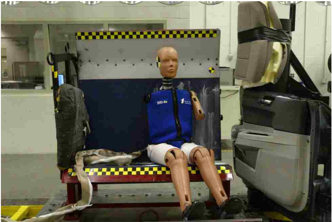
Figure 4-1: Heidelberg buck pole sled test set-up. [36].
