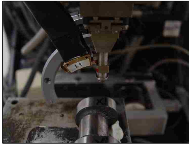
Figure 3.6 The measurement of residual stress using X-ray diffraction method
