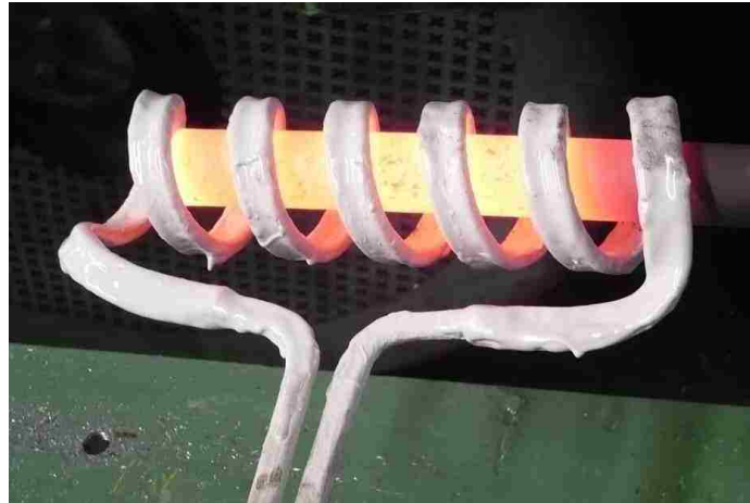
Figure 2.10 A conventional induction heating system consists of a cylindrical steel bar surrounded by a multi-turn induction coil [27].
