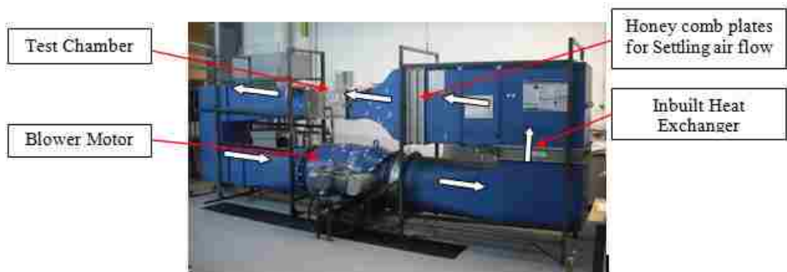
Figure-4. 10: Winds Tunnel with Blower Motor
