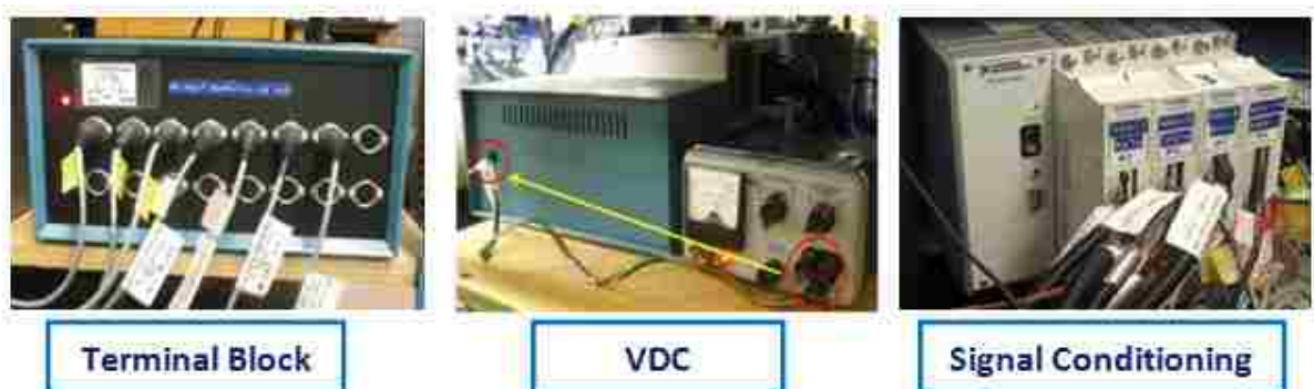
Figure-4. 18: Terminal Block, VDC and the Signal Conditioner
