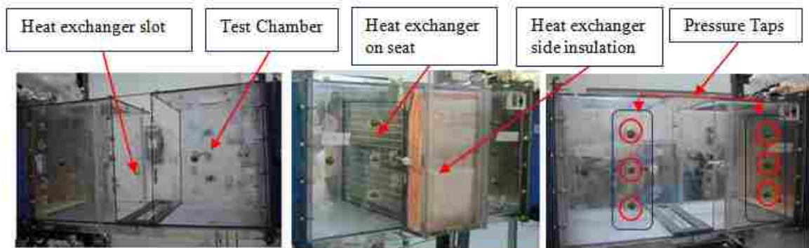
Figure-4. 11: Test Chamber and the Heat Exchanger
