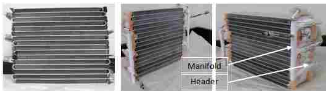
Figure-4. 21: Heat Exchanger Slab and the Manifold
