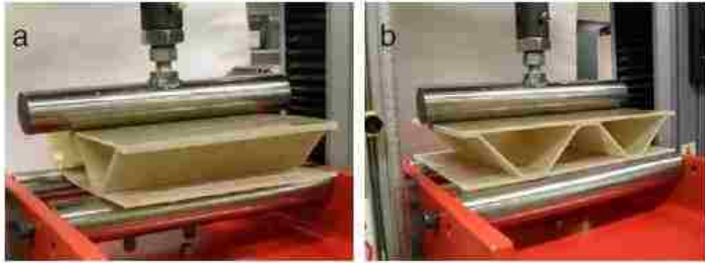
Figure 32: Three points bending tests on the corrugated sandwich composite coupon [64]
