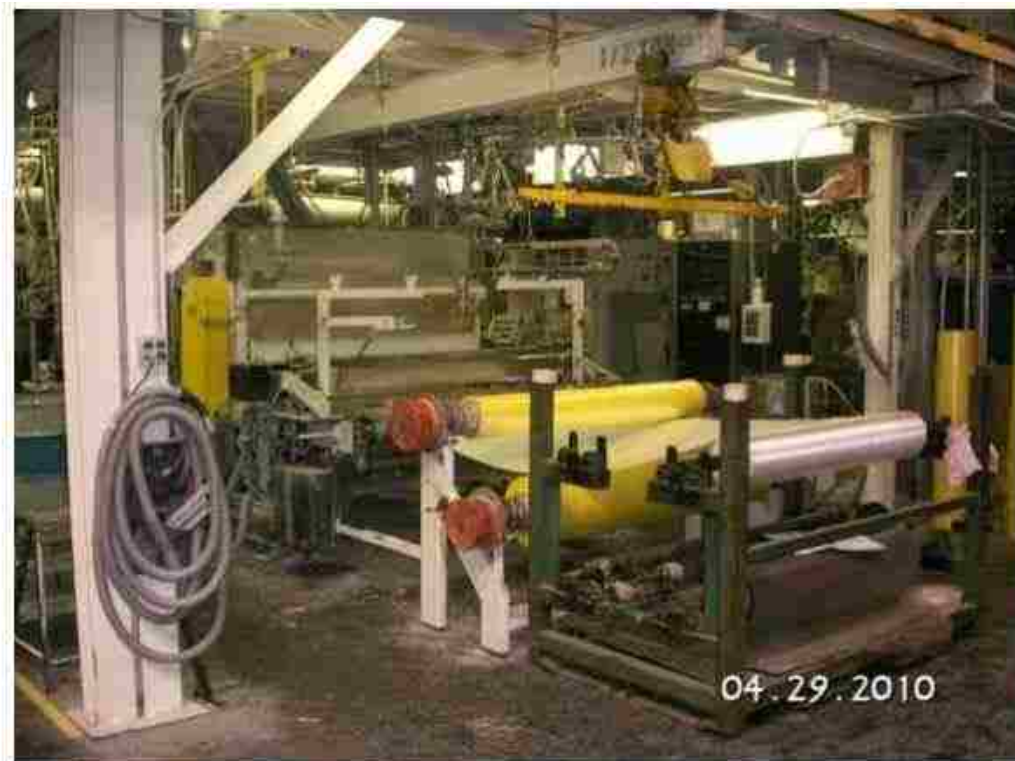
Figure 8: Fabric Mat being fed into SMC Compounder at CSP in Van Wert, Ohio
