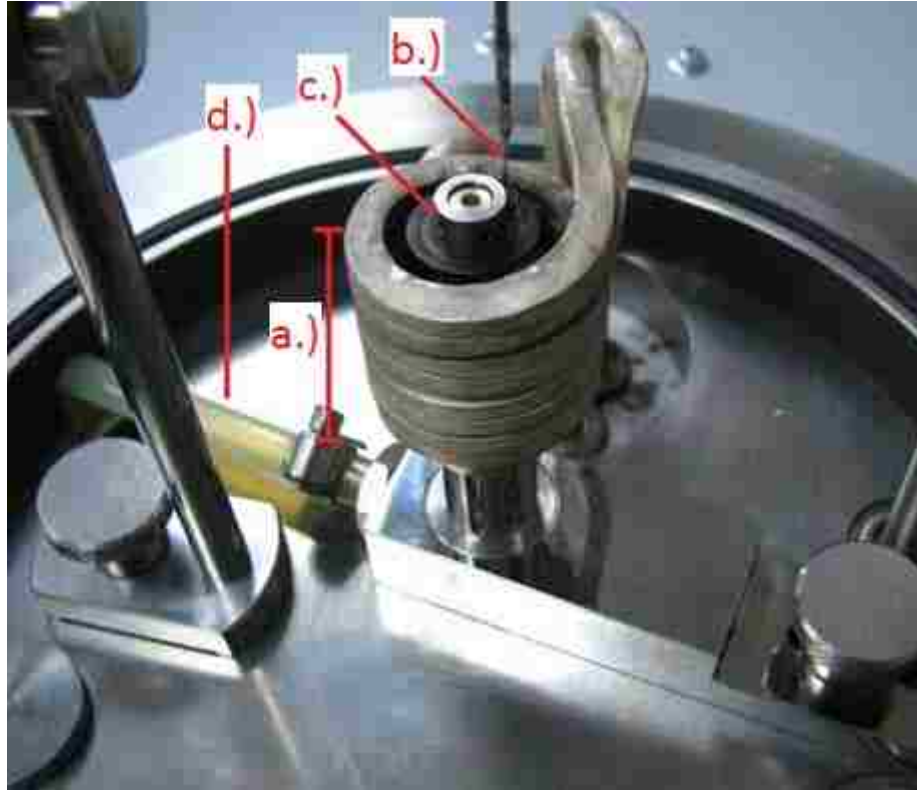
Figure 13 - Experimental setup for a hollow sample using compressed Ar cooling.
