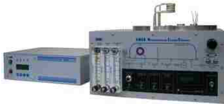
Figure 11 - Photograph of the UMSA Technology Platform (power supply and environmental chamber).
