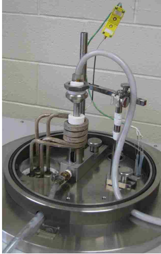
Figure 14 - UMSA configuration for rapid liquid quenching.
