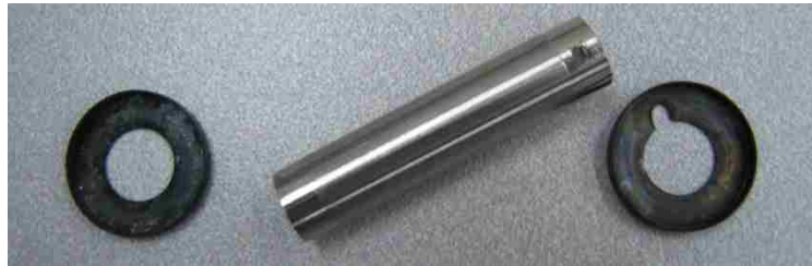
Figure 12 - End caps and centre tube for UMSA sample isolation.
