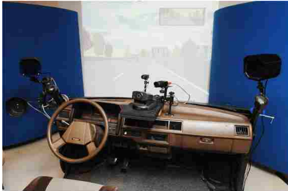
Figure 4.1: Setup of Driving Simulator at l'Université Laval, Photo Courtesy [39]
