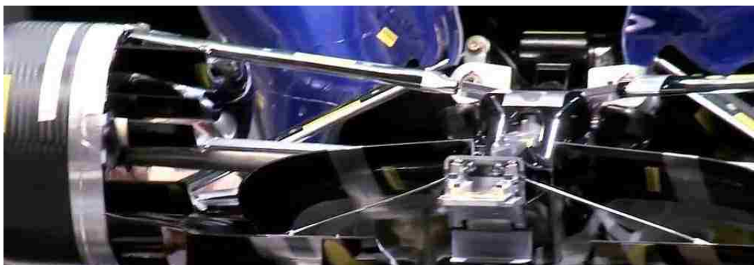
Figure 28: Example of F1 scale model suspension mounting points on the model spine (Screenshot taken from referenced video) (Williams in 60 seconds: Wind Tunnel, 2012).
