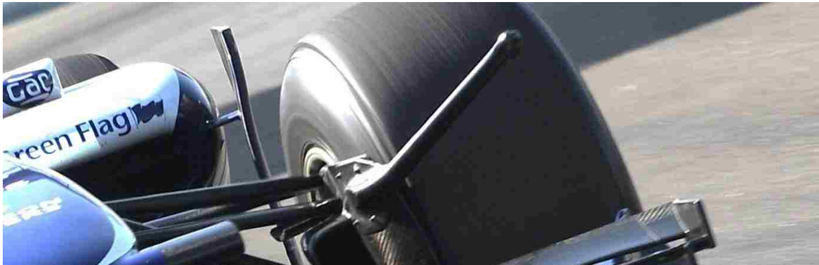
Figure 13: Williams F1 external measurement boom (Scarborough, 2010).
