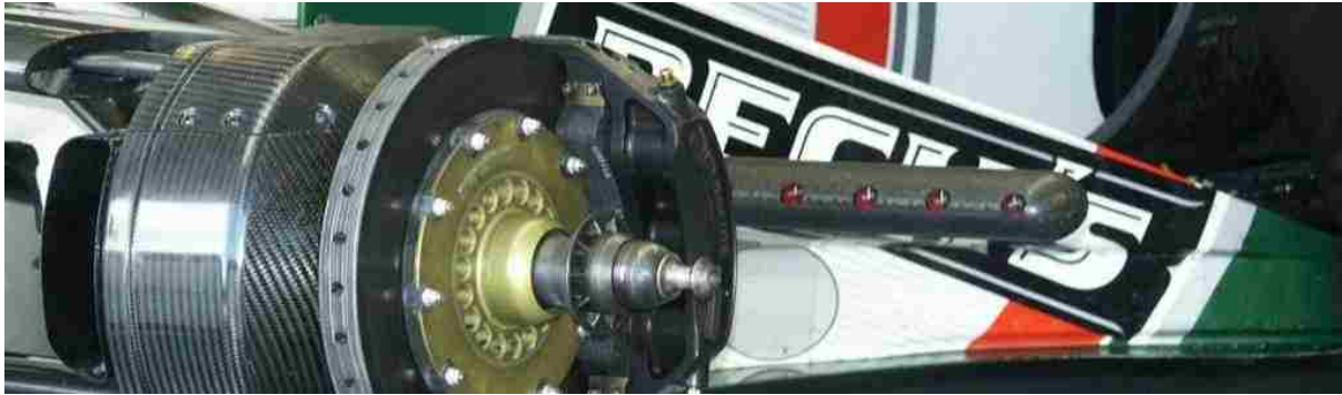
Figure 12: 2002 Jaguar F1 infrared sensor boom (Scarborough, 2010).
