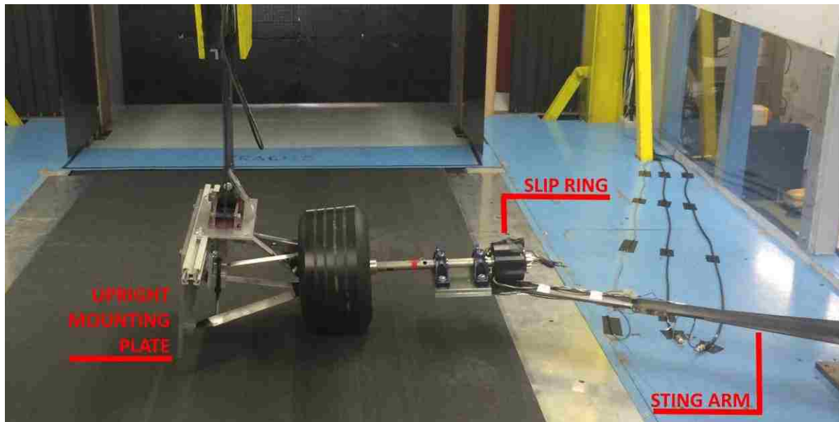
Figure 33: Wind tunnel test configuration using existing sting arm mount and custom upright mounting plate.
