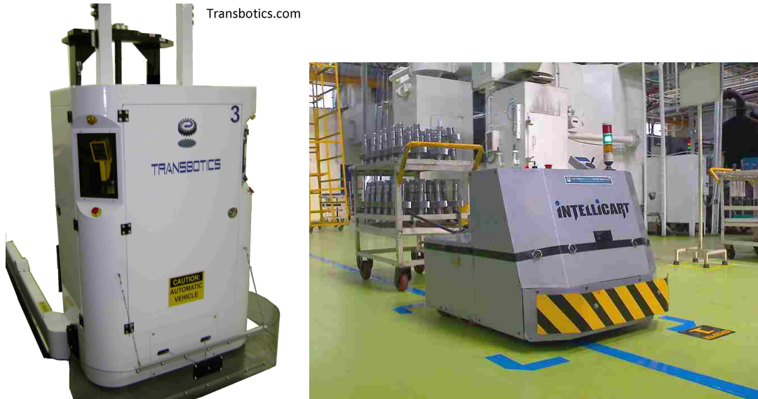
Figure 4: Examples of AGVs: an outdoor laser-guided vehicle on the left, and an indoor vehicle following a magnetic strip on the factory floor on the right
