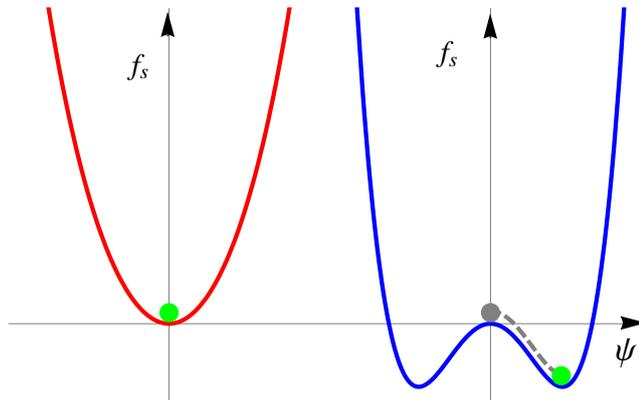
Figure 1.1: Plots depicting the free energy,  $f_s$ , as a function of  $\psi$  as described by (1.3). The left and right plots show  $f_s$  for  $\alpha > 0$  and  $\alpha < 0$  respectively. One can see that as  $\alpha$  drops below zero new minima appear at non-zero  $\psi$ .
