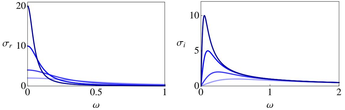
Figure 1.2: Plots showing the real,  $\sigma_r$ , and imaginary  $\sigma_i$  parts of the conductivity as a function of  $\omega$ . Here  $\omega$  is the frequency of any applied electric field given by  $\mathbf{E} = E e^{i\omega t} \mathbf{e}_x$ . The darker lines correspond to larger relaxation time,  $\tau$ .
