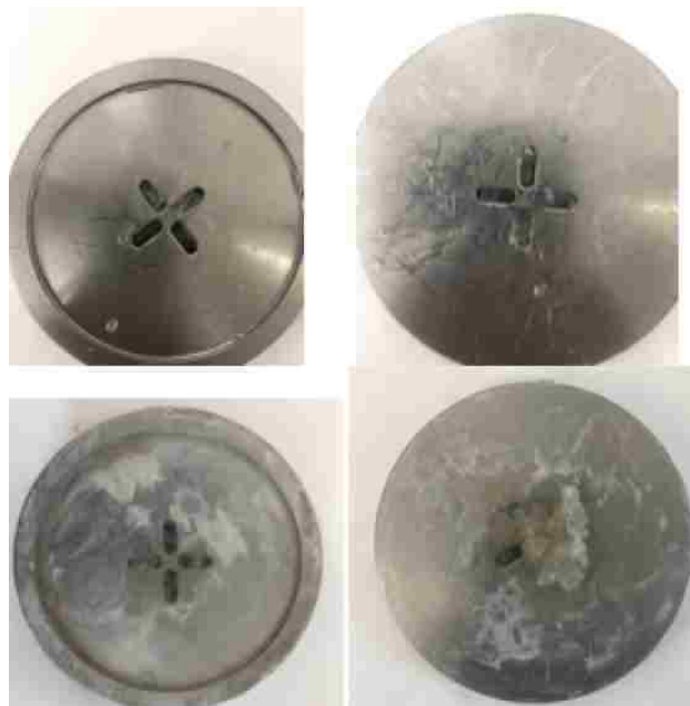
Figure 5.13. Slot disc sealed with 0.24 lb/gal of LCMs (top) versus 0.48 lb/gal bottom
