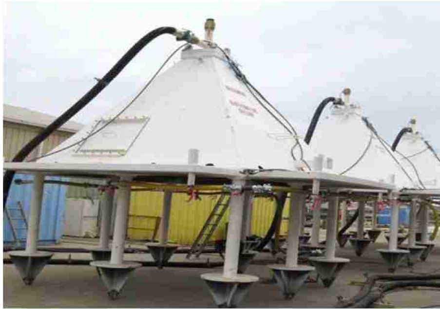
Figure 57: Cone shaped collector used in oil suction on Taylor Energy’s buried platform (from RRT-6)
