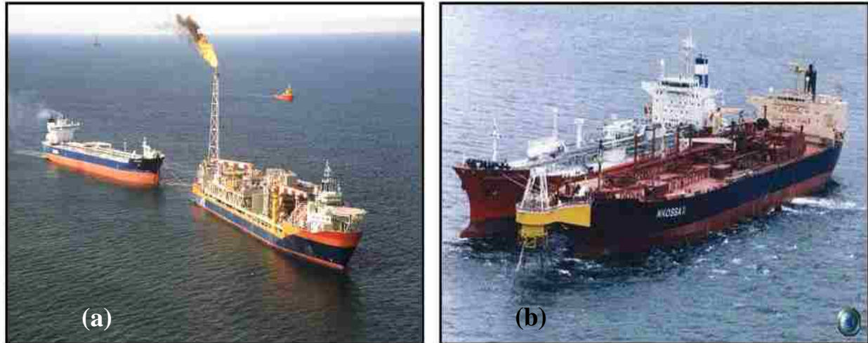
Figure 38: (a) Tandem and (b) side by side offloading from FPSO (From Regg-2000)
