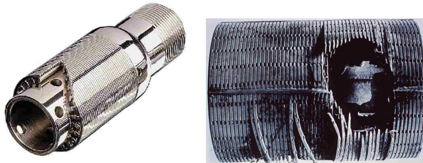
(a) Dual screen mesh (source: Hole Products, Inc.) (b) Erosive damage due to fines migration (King, 2009)
