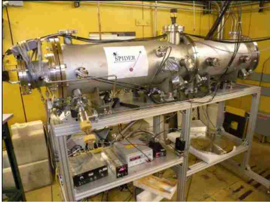
Figure 17: Current LANL SPIDER 2v -2E chamber, the target is in the center.
