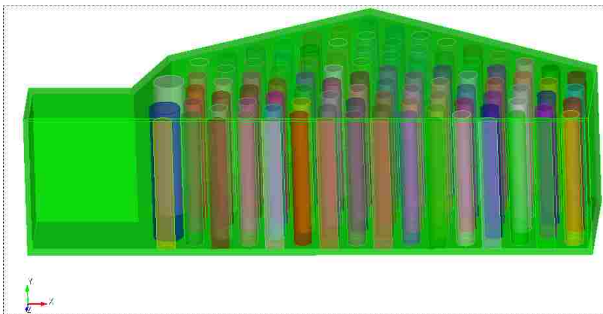
Figure 35. Side View of the Fuego LP Model with Support Posts and Swirl BCs.
