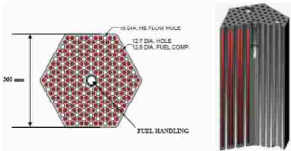
Figure 12. Hexagon Block Cross-Section [INL, 2007].
