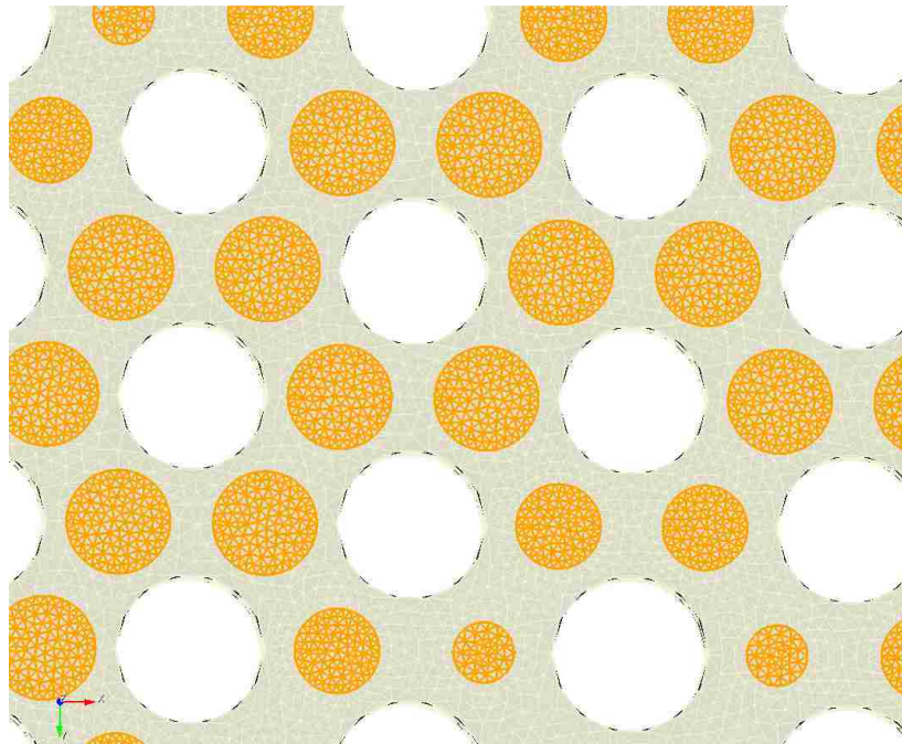
Figure 38. Zoom of the Fine Mesh Showing Resolution for the Small, Medium, and Large Jet Channels.
