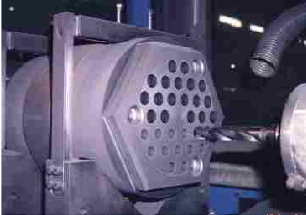
Figure 13. Hexagon Block Being Machined [Burchell, Bratton, Windes, 2007].
