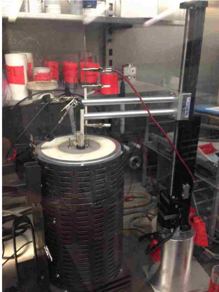
Figure 8-Experimental Setup featuring a high temperature Kerr furnace, electrodes, and vertical translator
