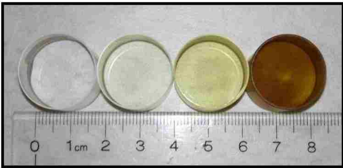
Figure 5.6.6: Image of unirradiated and irradiated CaF 2 crystals. Unirradiated on left and irradiated organized from left to right with least to most irradiation.
