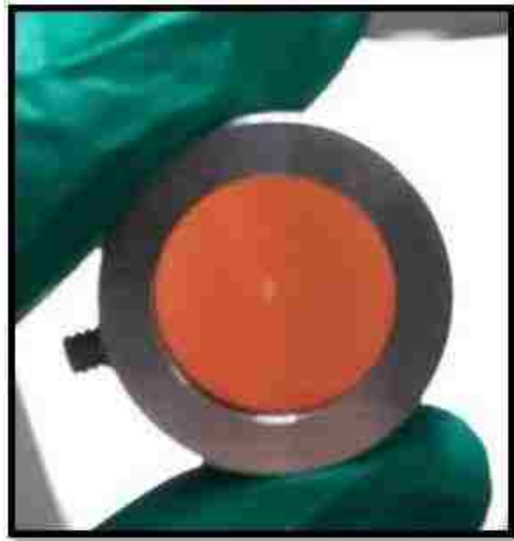
Figure 5.6.2: Demonstration of the "bleaching" effect that occurred after attempting to mode-lock the cavity with this FPE inserted.
