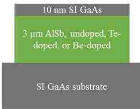
Figure 27. R14-145, R14-171, R14-172, R14-175, R14-176, R14-177, R14-178, R15-34; AlSb structure used for Hall measurements.
