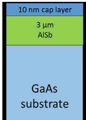
Figure 48. AlSb doping study sample structure.
