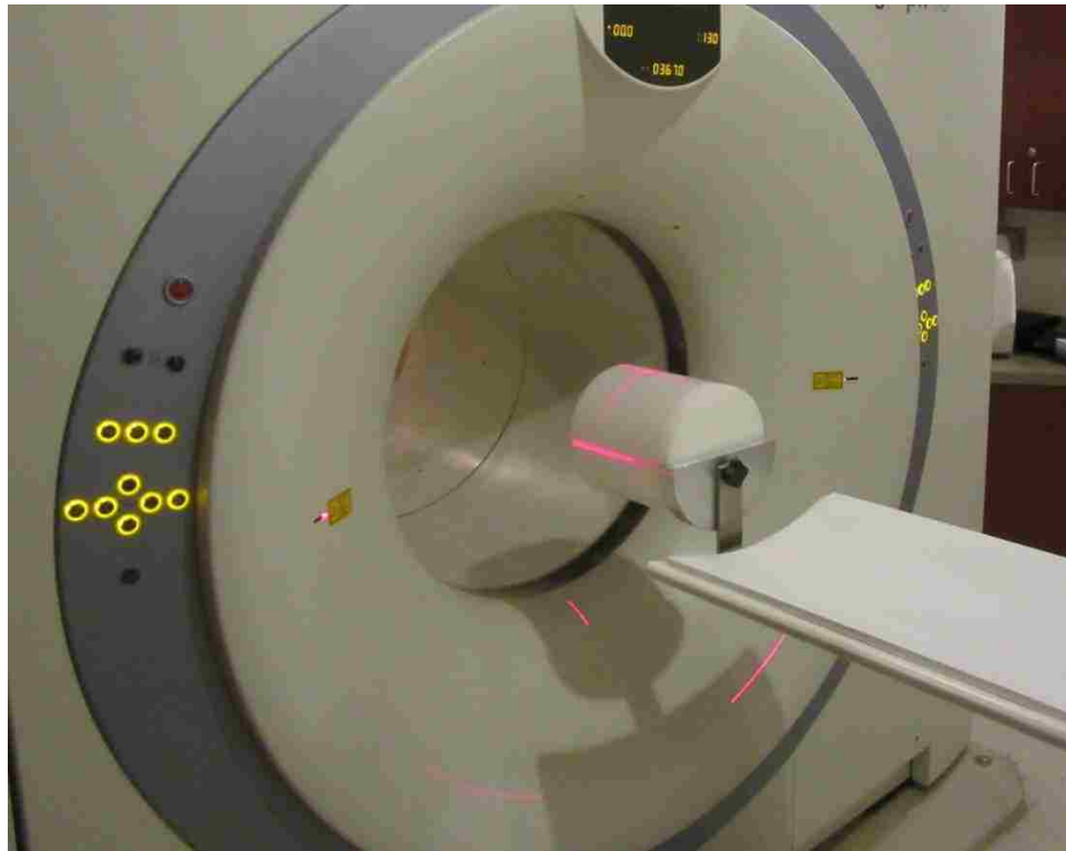
Figure 48: Cylindrical uniformity phantom mounted on bracket at end of patient table. The uniformity phantom is used for quality control of the PET/CT scanner. Phantom volume is 6.283 liters. Scanner is a Siemens Biograph 16 PET/CT.
