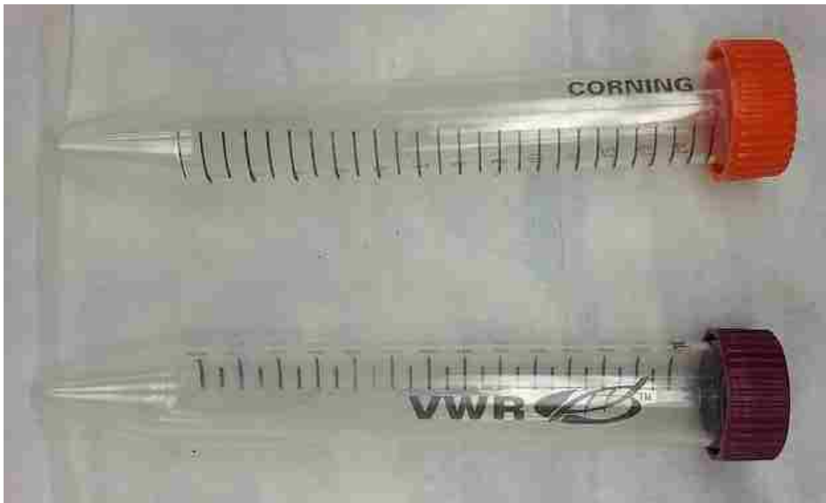
Figure 11: Two different models of 15 mL polypropylene centrifuge tubes used in these radiolabeling experiments.
