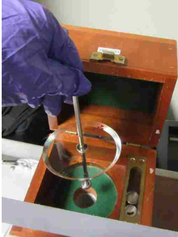
Figure 60: Amersham SIA.20 Sr-90/Y-90 ophthalmic applicator being withdrawn from its case. The source is the disk at the end of the rod.
