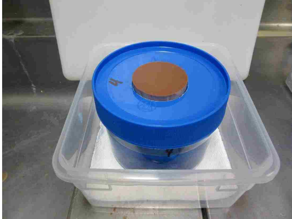
Figure 64: Phantom completely assembled. The solid water plug and film are in place. The final step in deployment of the phantom is to invert the entire assembly.
