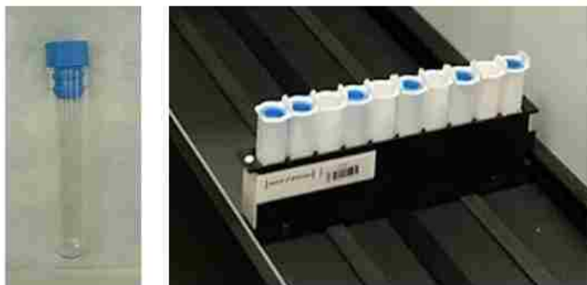
Figure 12: PerkinElmer sample vial (left). Vials in rack ready for counting in Wizard 2 counting system.
