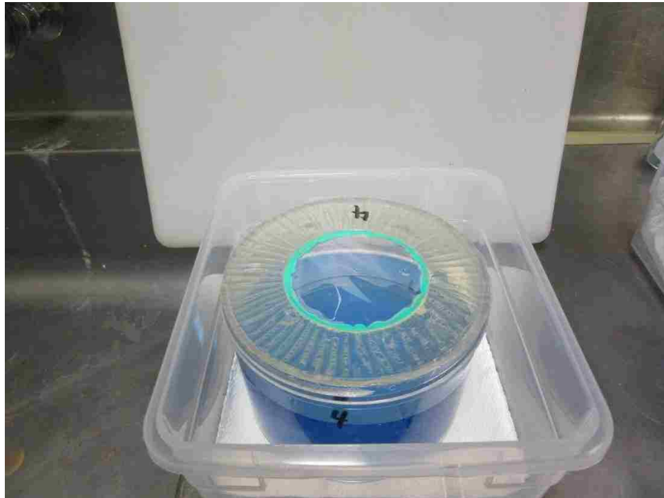
Figure 62: Phantom 4 with lid off showing the support ring and 0.001" thick polyester beta-window. The phantom contains 400 mL of fluid and blue food coloring. Silicone grease is used to seal the support ring and body of phantom.
