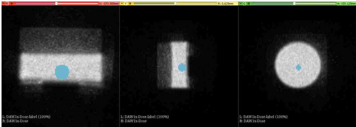
Figure 76: Tomographic absorbed dose map output from GATE run. A total of 10^7 primary Y-90 electrons were used. A VOI shown in blue was used to determine the absorbed dose to the water in the central region of the phantom.
