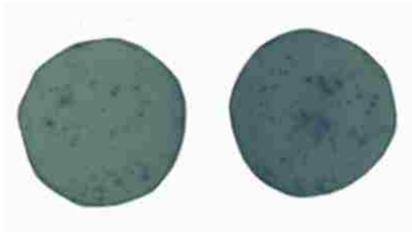
Figure 83: Film disks D1 and D3. Dark spots are present across the entire area of the film. This indicates the presence of localized spots of high activity on the beta window.
