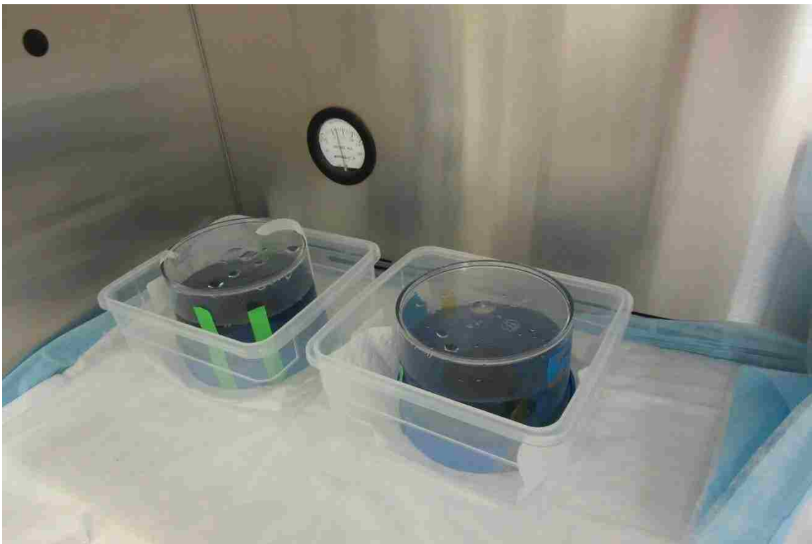
Figure 70: Phantoms 4 and 2 in the inverted position. Each phantom had the radiochromic film and solid plug on the underside.
