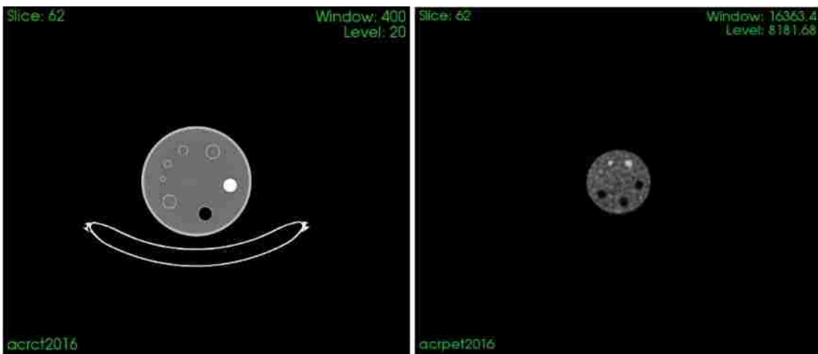
Figure 54: Side by side comparison of CT (left) and PET (right) of slice 62 through ACR PET phantom.
