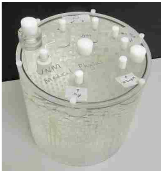
Figure 50: The ACR PET phantom. The lid contains objects that enable measurement of the imaging capability of a PET/CT scanner. A positron-emitting radionuclide is added to the bulk fluid in the phantom and also to the ‘hot’ cylinders in the lid. The hot cylinder-to-bulk contrast ratio is 2.5:1
