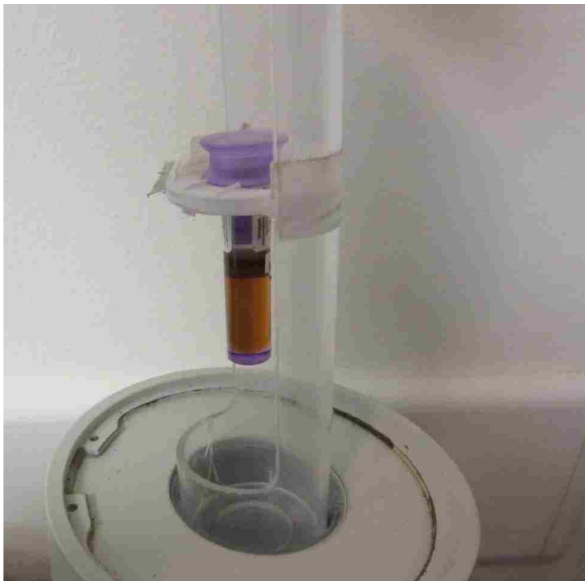
Figure 8: Calibration source for F-18 in a dose calibrator dipper. The dipper is partially in the well of the dose calibrator ionization chamber. The source is NIST-traceable with a known activity of Ge-68/Ga-68. Gallium-68 is a positron emitter. The Ga-68 activity is converted into NIST-traceable activity for F-18.
