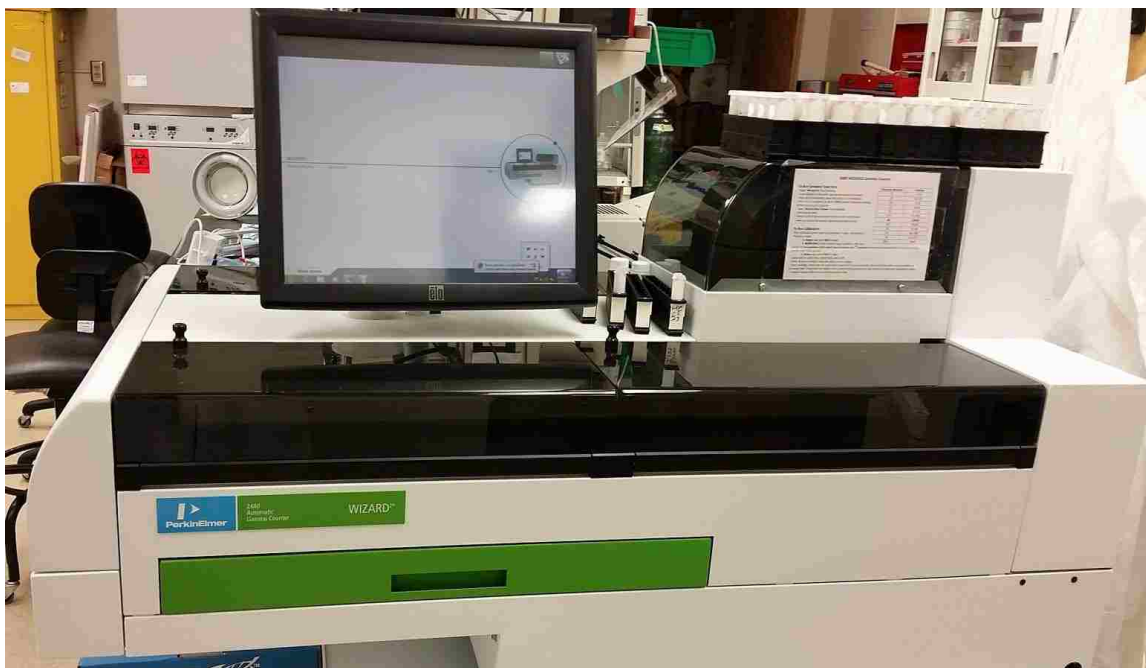
Figure 9: PerkinElmer "Wizard 2 " model 2480 automatic gamma counter.
