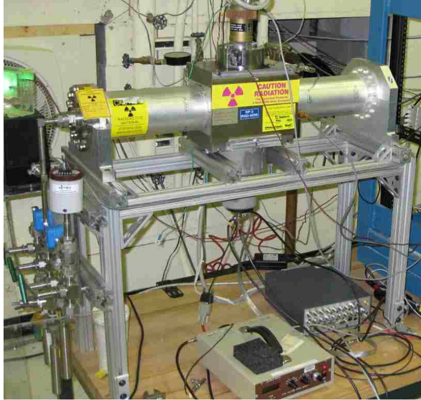
Figure 3-8: Large horizontal \text{UF}_6 source with three pipe thicknesses, variable gas pressure, and variable enrichment. The active system is mounted on the pipe with the x-ray tube on the top pointing downwards; the \text{LaBr}_3 detector is mounted on the bottom in its tungsten composite shielding.
