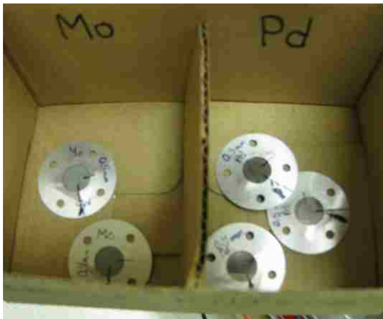
Figure 3-5: Some of the molybdenum and palladium notch filters attached to their mounting rings.
