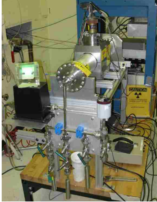
Figure 5-4: Refurbished horizontal source. Shown are the new ½” diameter pipes and the two bottles of \text{UF}_6 (foreground, bottom). The bottle on the right is empty.
