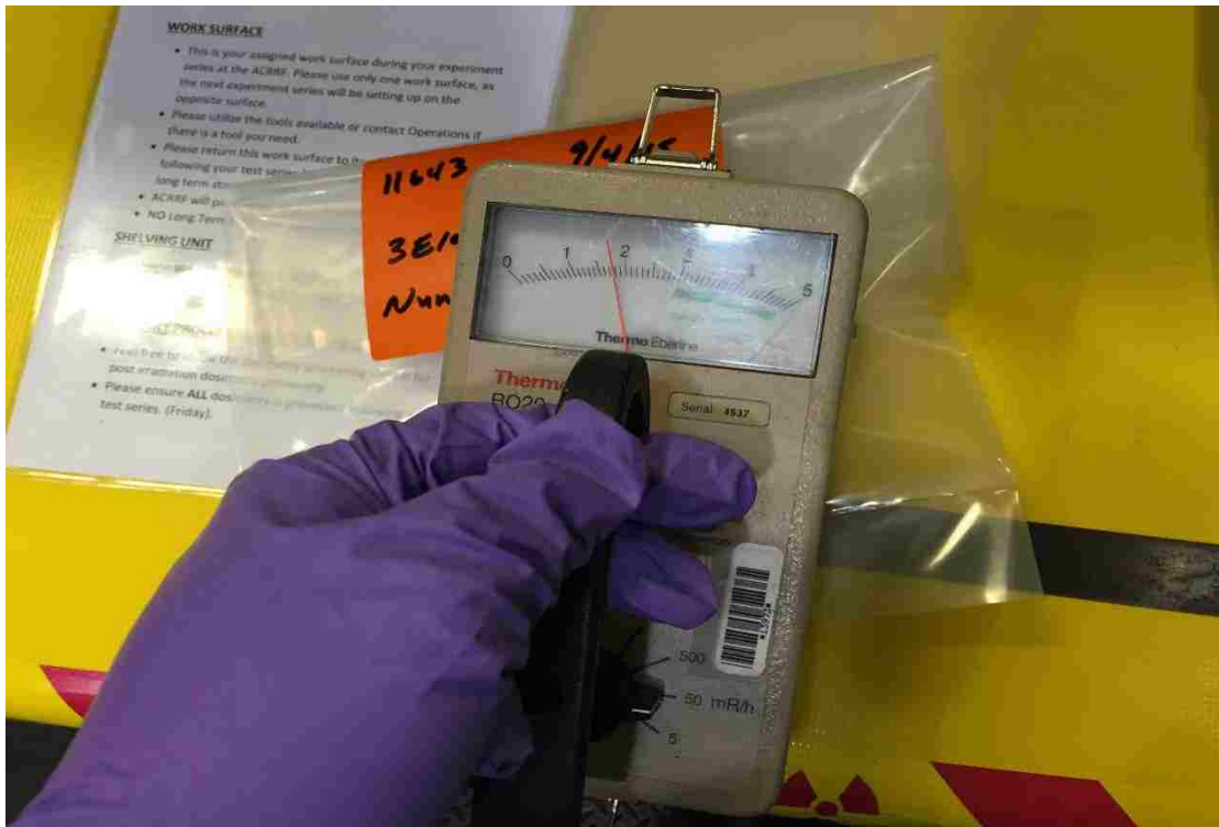
Figure 17 - Example of On-Contact dose rate measurement
