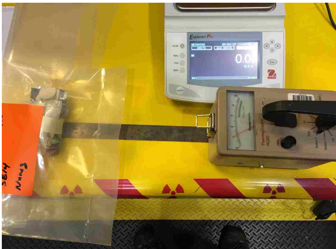
Figure 18 - Example of 1-foot dose rate measurement
