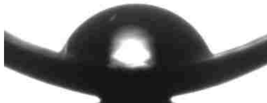
Figure 2.3 Contact angle measurement of SS316 (0.508mm) as-received inner surface
