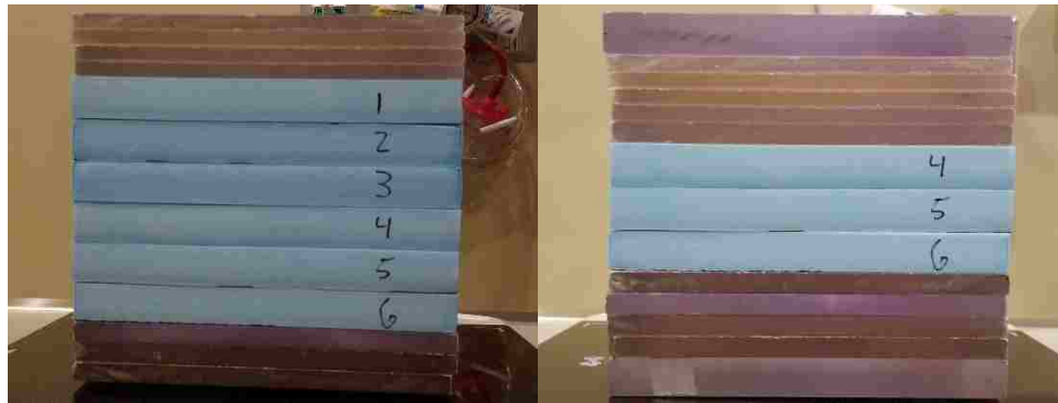
Figure 4-8: Inhomogeneous phantom setup. "Large" phantom on the left consists of 16 cm of Styrofoam (blue blocks) and 8 cm of polystyrene (clear blocks). "Small" phantom on the right consists of 8 cm of Styrofoam and 16 cm of polystyrene.
