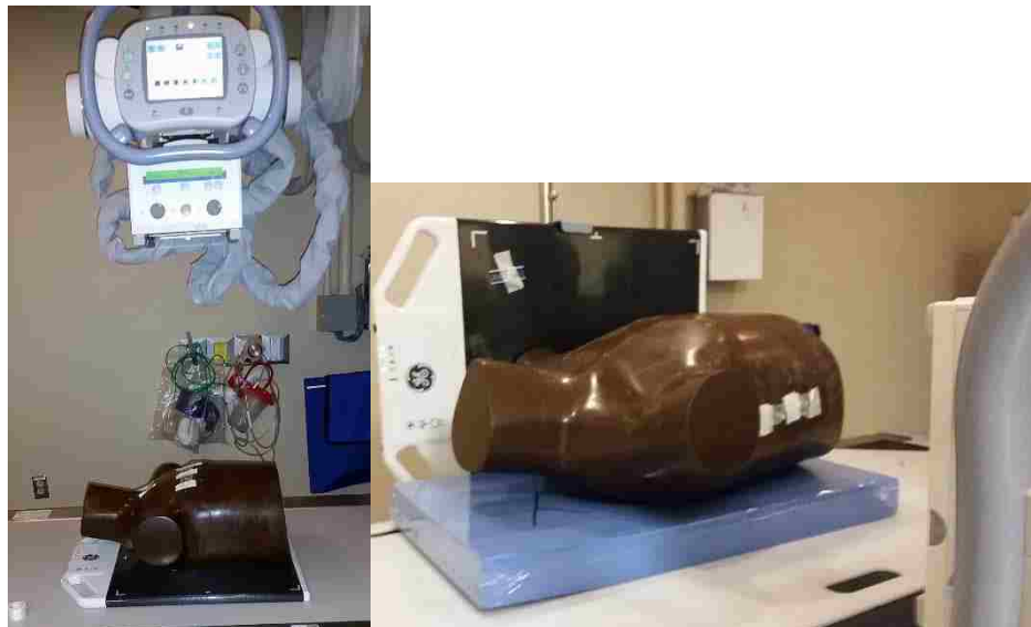
Figure 5-2: Clinical setup of the Alderson chest phantom for AP and Lateral radiographs. For the lateral radiograph, a radio transparent pad was placed underneath the phantom in order to lift it off the table and prevent any table artifacts in the image.
