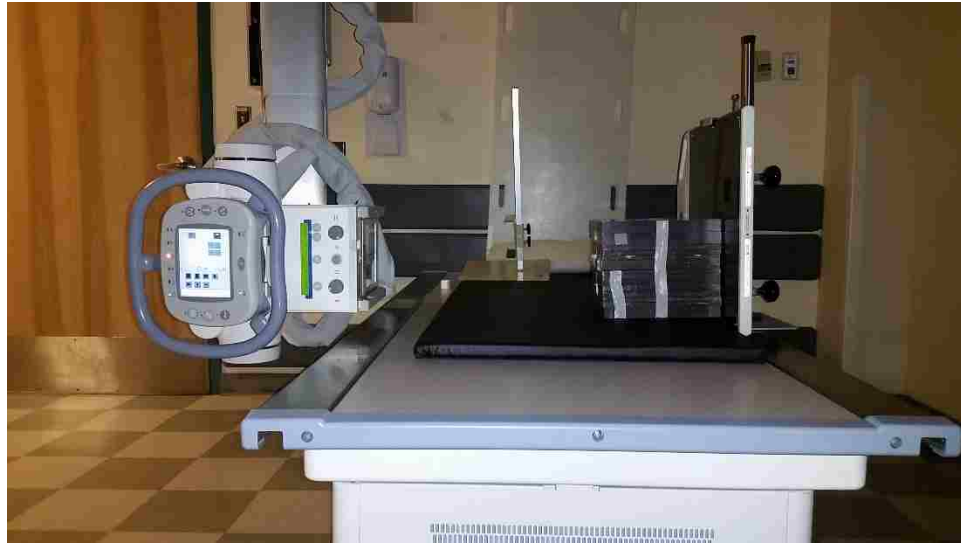
Figure 3-11: Lateral setup for nanoDot measurement on polystyrene phantom.
