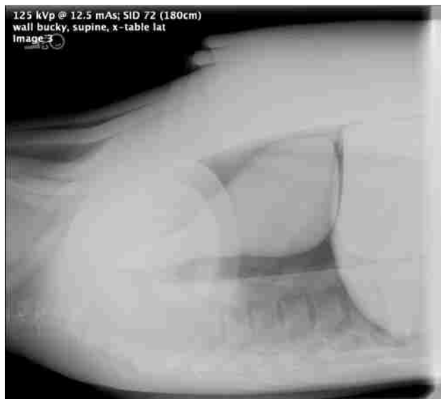
Figure 5-5: AP and Lateral radiographs of the anthropomorphic phantom with 5cm of Super-flex added.
