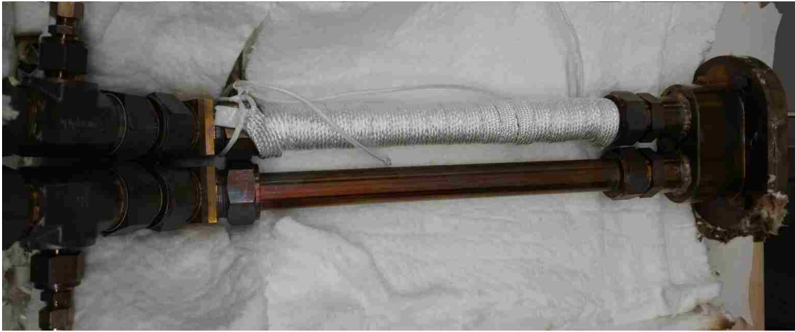
Figure 3-25 Post salt shakedown test loop
