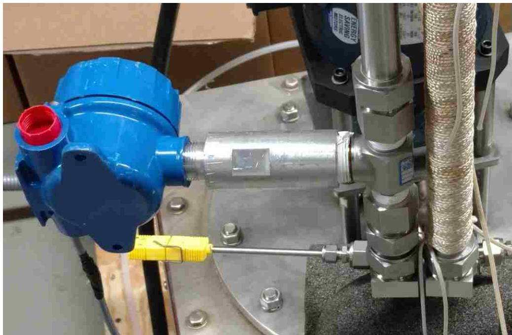
Figure 3-7 Omega FTB-1400 flow meter with signal conditioner
