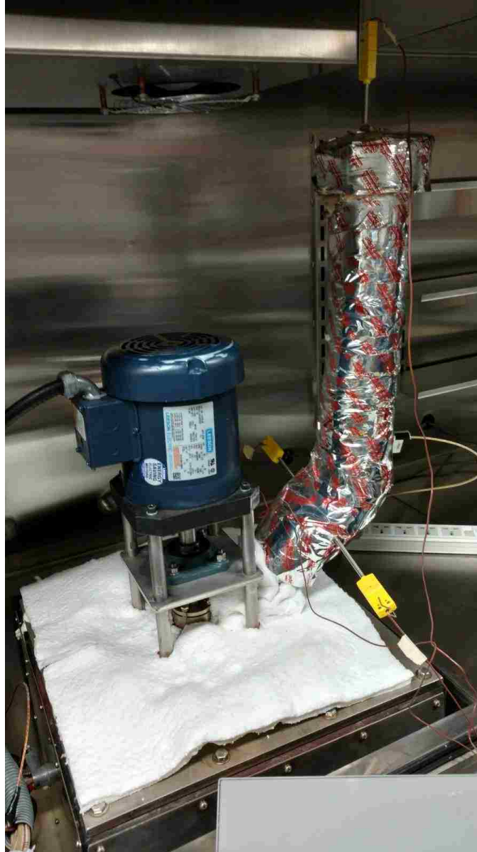
Figure 3-21 Test loop in salt shakedown configuration
