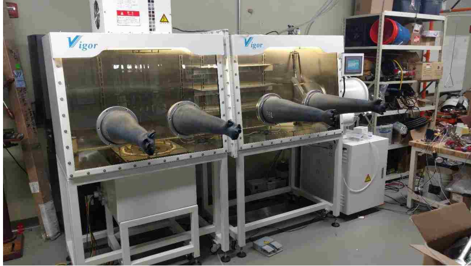
Figure 3-20 Fully Assembled Glovebox
