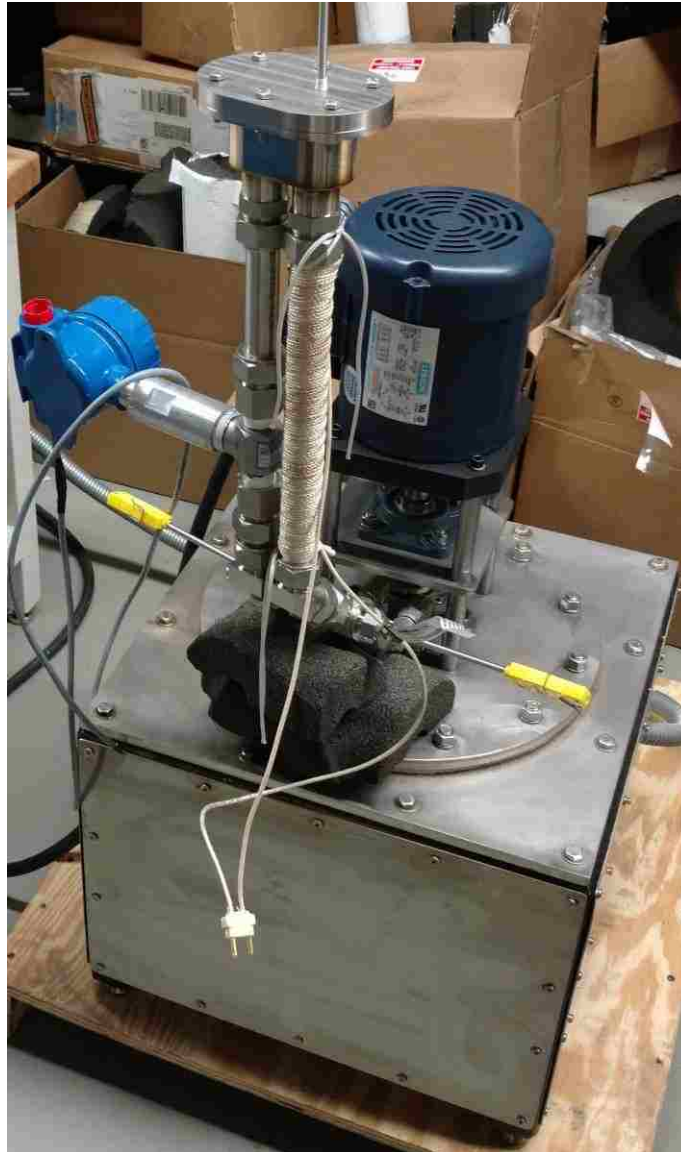
Figure 3-11 Pump and Melt Tank
