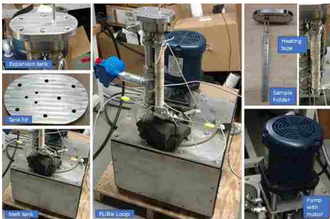
Figure 3-18 FLiBe loop and component pictures
