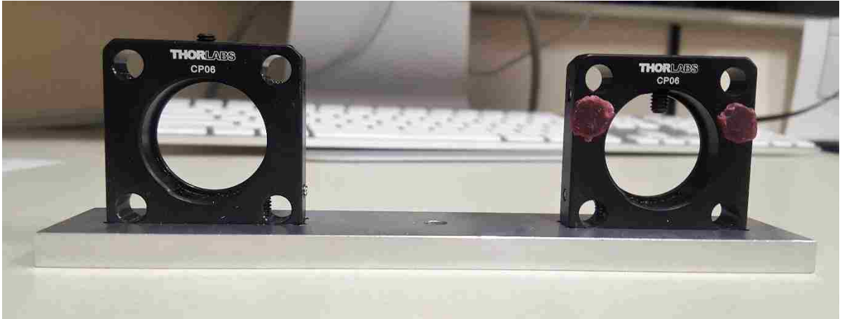
Figure 17. An image of the custom mount made for the spectrophotometer measurements.
