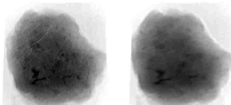
Figure 1.4: Image quality degradation due to demagnetization over the course of a tomography run on a meteorite [11]. Images are the same view of the object; note blurring and substantial loss of fine details in right image.
