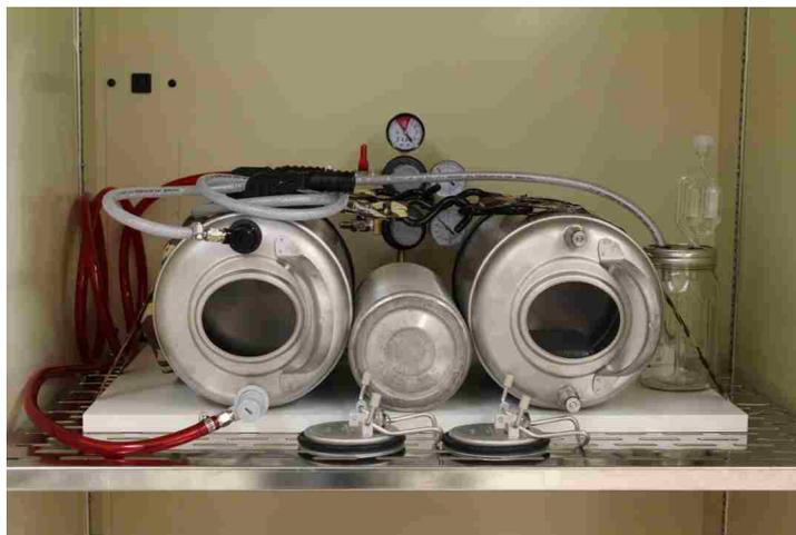
Figure 3.1: **High pressure anaerobic incubation chamber.**
