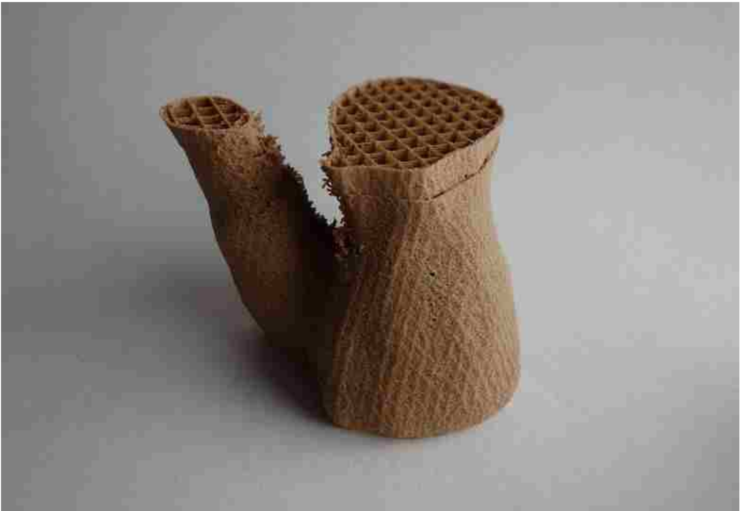
Figure 37: 3-D printed segment of straw core.
