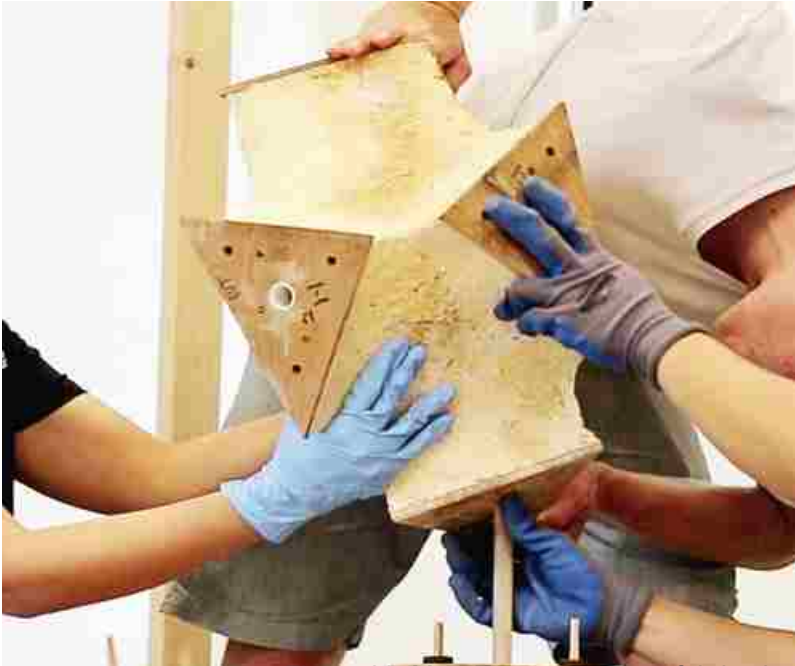
Figure 29: MycoTree component fabrication
