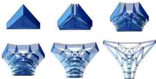
Figure 27: MycoTree polyhedral structural form diagram
