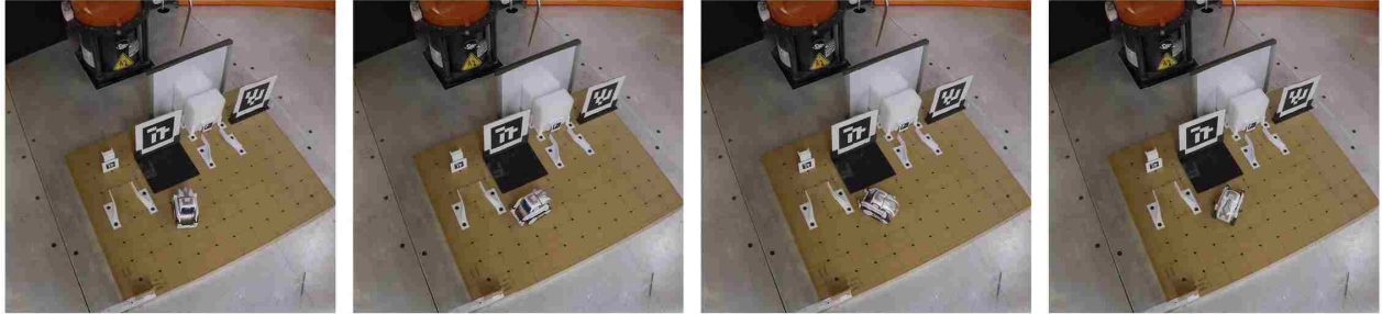
Figure 23 The mobile robot looks for the locations of pre-defined AR tags
