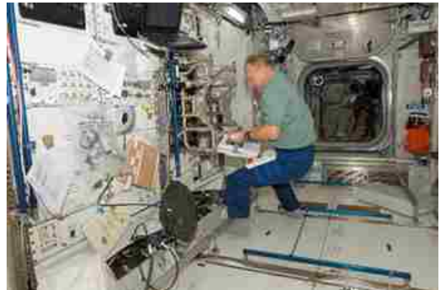
Figure 5: International Space Station (Handles placed throughout the station allow for astronauts to grip and orient themselves to any surface)
