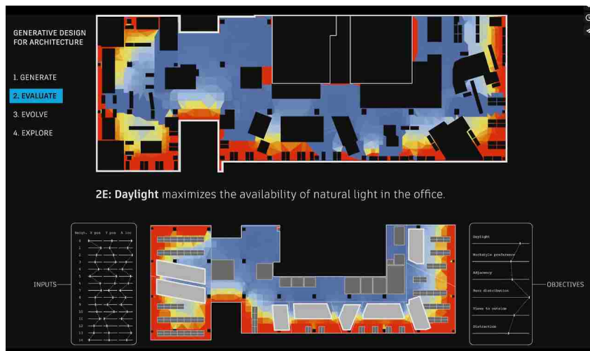
Figure 5: Generative Design Method (A daylight evaluation done during the generative design process used to create the Autodesk MARs office)
