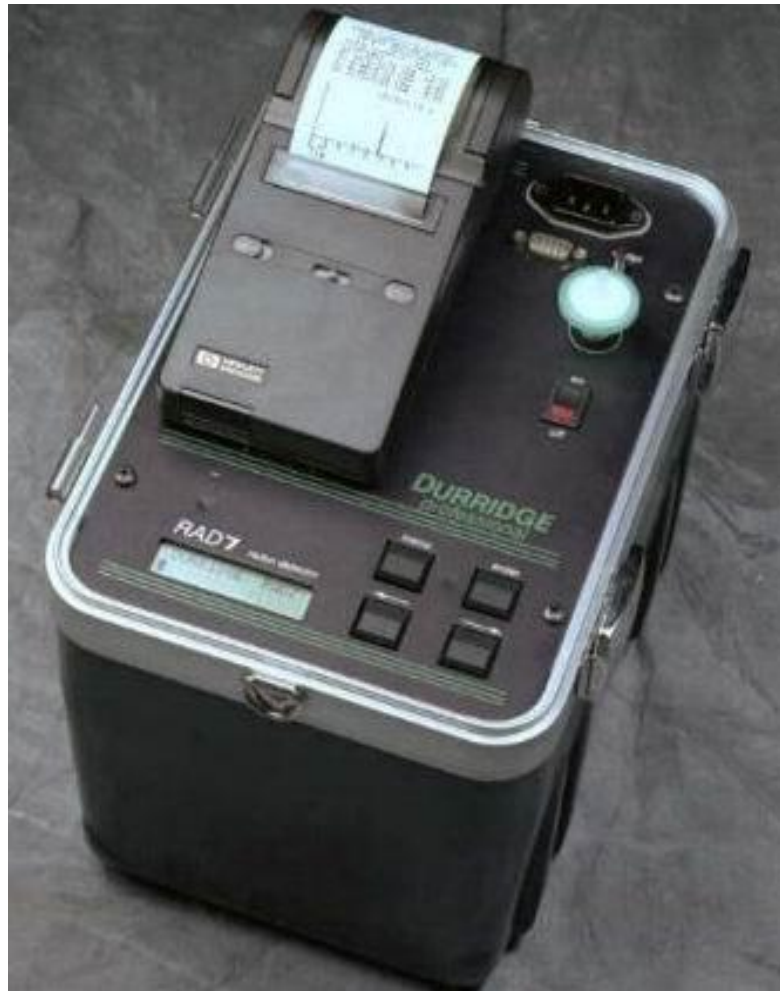
Figure (2.2): The DurrIDGE RAD7 electronic continuous radon monitor with a HP printer mounted for immediate printing of results (DurrIDGE Co., 2012).
