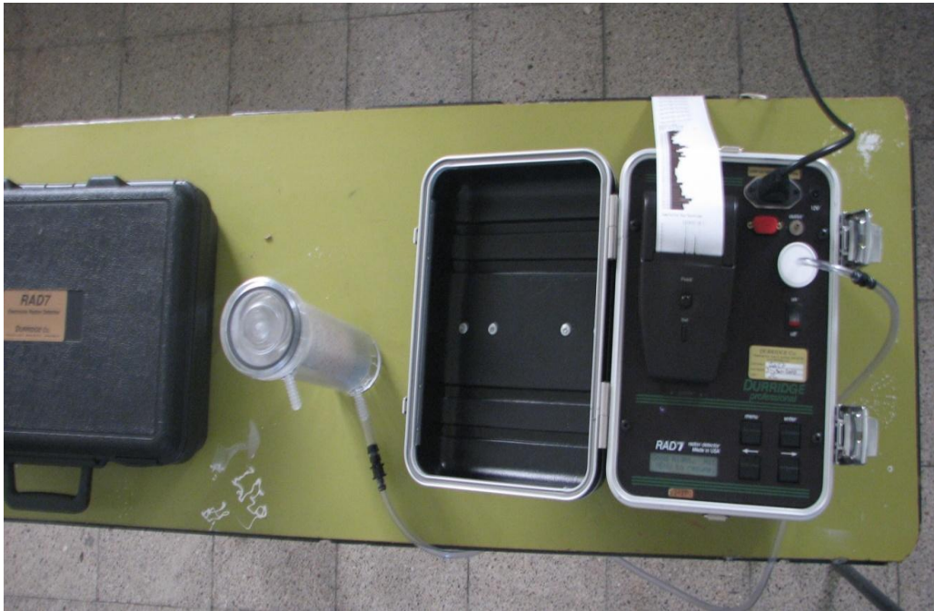
Figure (4.2): Measurement apparatus RAD7
