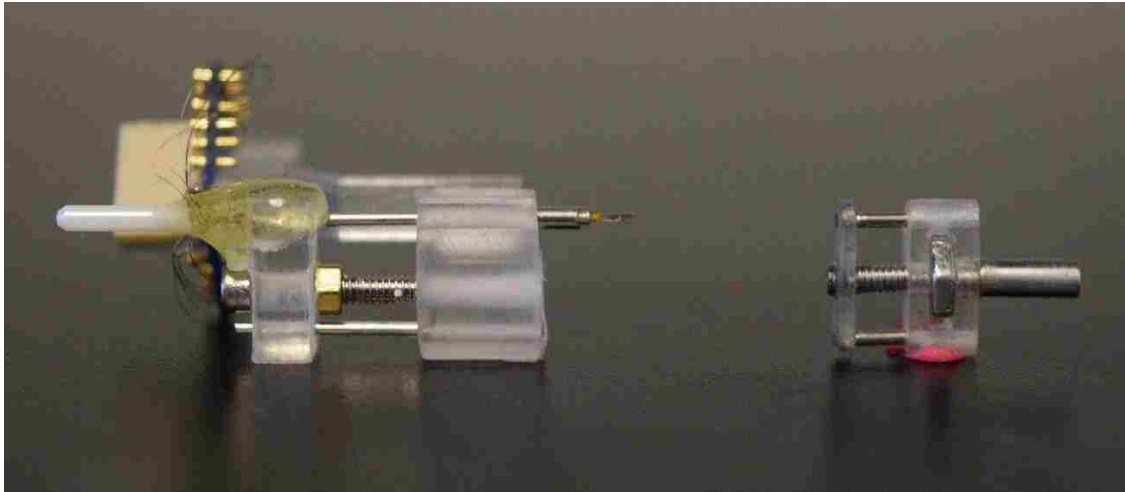
Figure 15: Comparison Between New and Previous Device – Side-by-side comparison of the previous device (Left) to the new device (Right) showing significant reduction in size for the new device. Note: This is an image of the new device without the fibers implanted or EIB attached which makes it appear smaller than the final implanted device would be.
