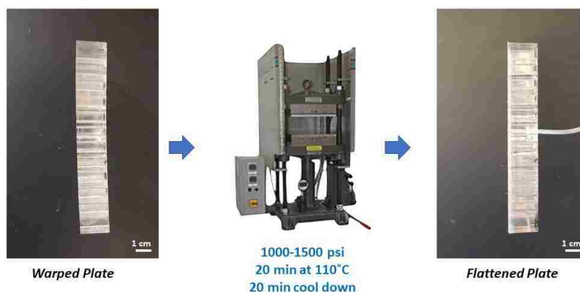
Figure 20: Thermal annealing process to remove well plate warping
