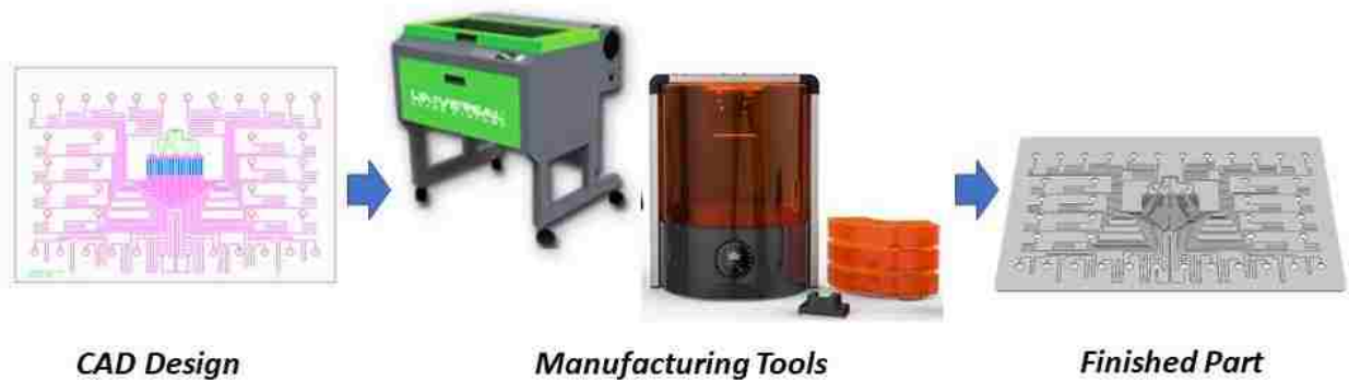
Figure 2: Digital microfluidic manufacturing process flow
