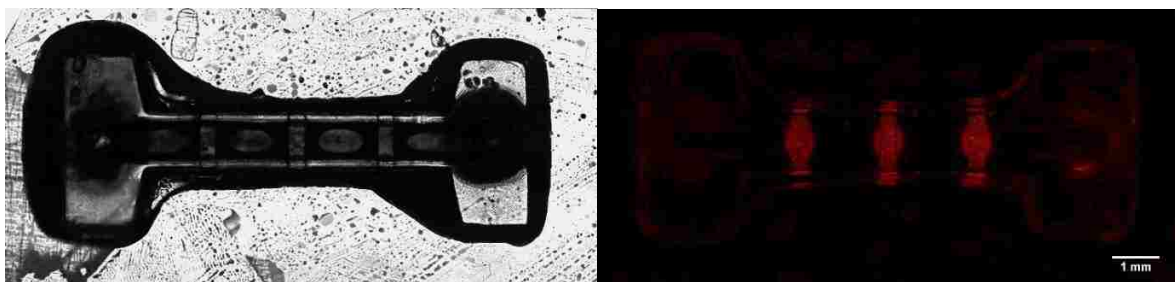
Figure 39: Brightfield and fluorescence image of 3D printed biosensor channel with entrapped avidin conjugated with Texas Red dye
