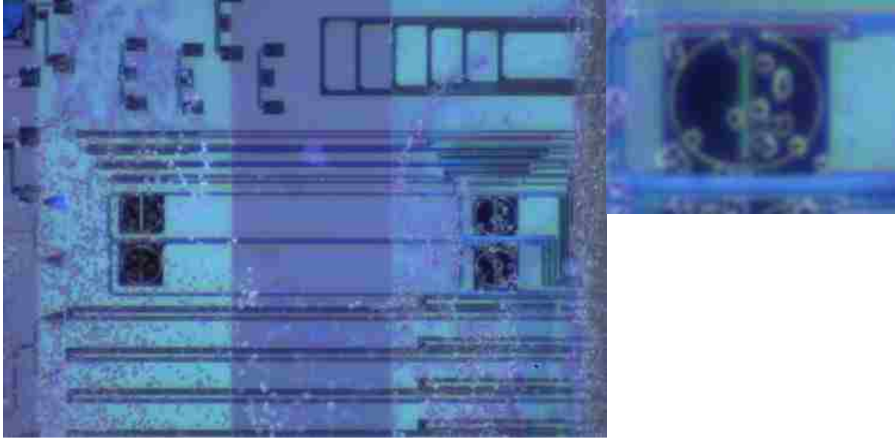
Figure 2-16 An overhead micrograph of the sensors during the forward typing assay. The flow was stopped for taking an image. (Inset) Magnified view showing the relative size of RBCs to an individual ring resonator.
